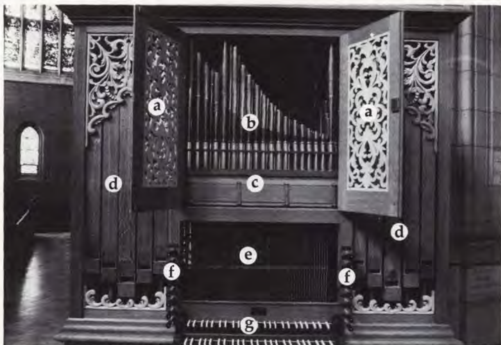
Small Flentrop organ (1976) in Trinity Cathedral, Cleveland, showing traditional components: a. Brustwerk doors; b. reed pipes; c. windchest; d. pedal pipes; e. tracer rods or trackers (direct mechanical connections between keys and pipe valves); f. stops (levers which admit or shut off air to various registers of pipes); and g. keyboards. (Photo: David Knipper)
