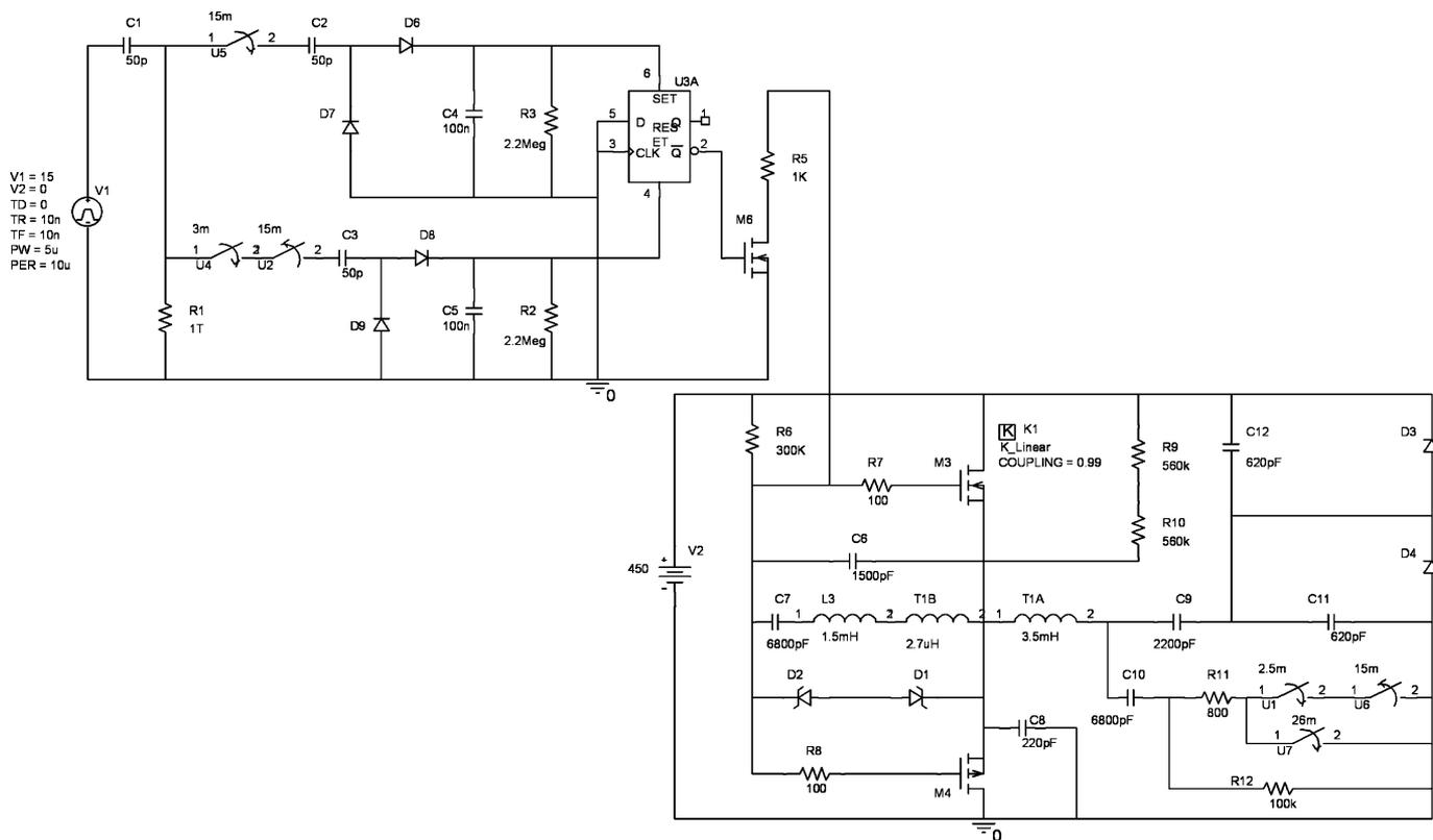
Fig. 11. PSPICE model of the proposed discrete dimming ballast.
