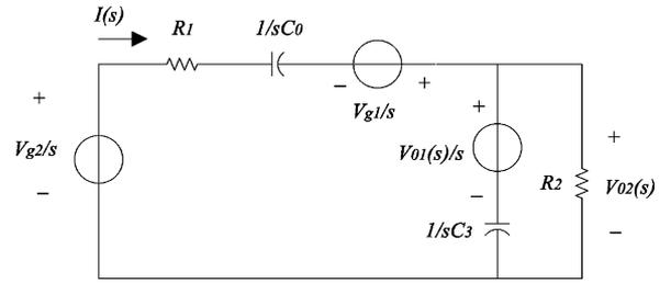
Fig. 8. Laplace transformed equivalent circuit in mode II.
