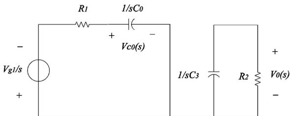
Fig. 7. Laplace transformed equivalent circuit in mode I.
