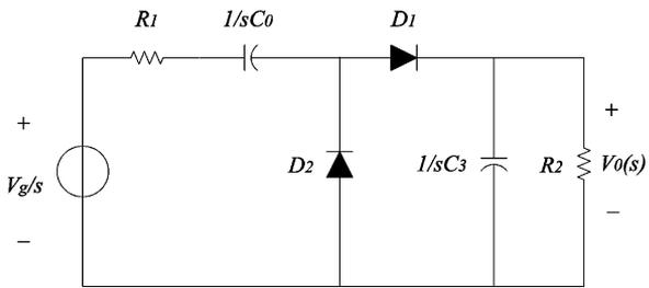
Fig. 6. Charge pump Laplace transformed equivalent circuit.
