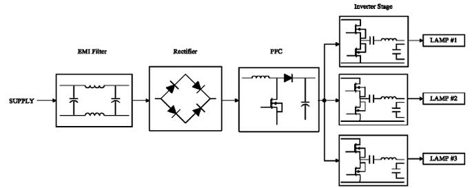
Fig. 2. Block diagram of the ballast module.
