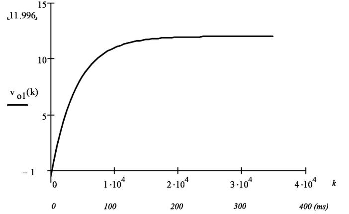
Fig. 10. Charge pump output voltage waveform (MathCAD result).
