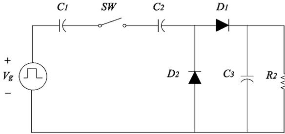
Fig. 5. Topology of the charge pump circuit.
