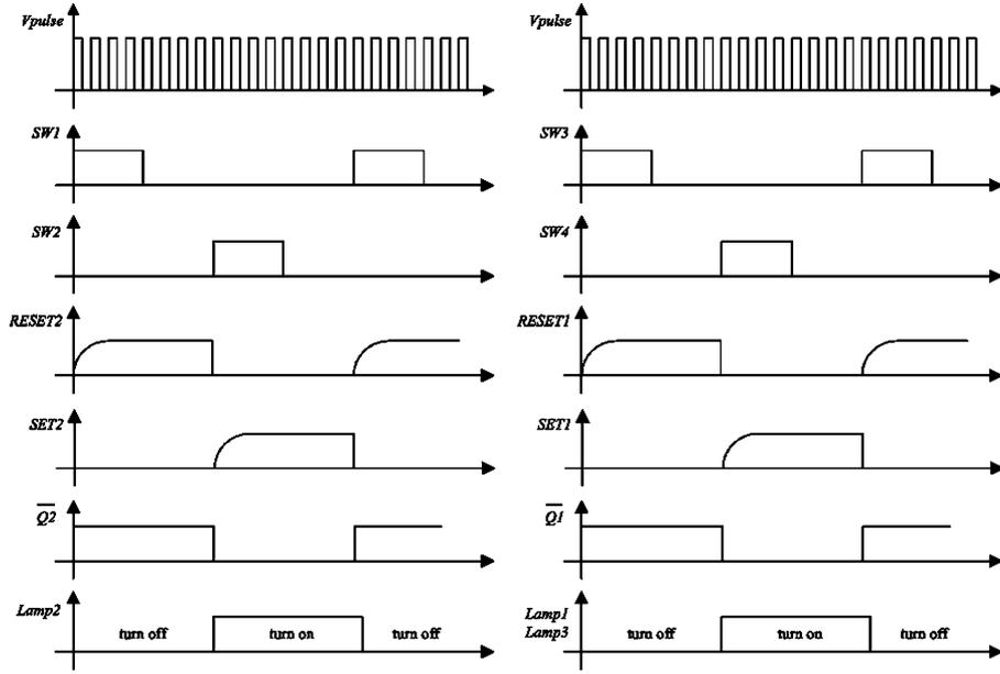
Fig. 4. Timing diagram of proposed digital dimming controller.
