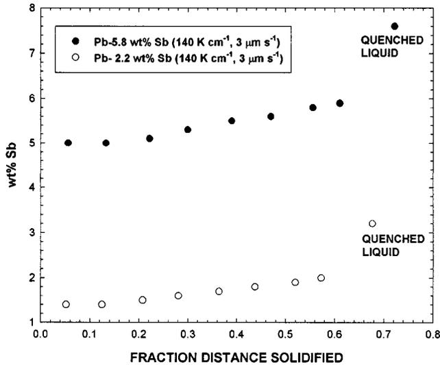
Fig. 1—Axial variation in antimony content due to macrosegregation in directionally solidified samples of Pb-2.2 wt pct Sb and Pb-5.8 wt pct Sb, grown at  $V = 3 \mu\text{m s}^{-1}$  and  $G = 140 \text{ K cm}^{-1}$ .
