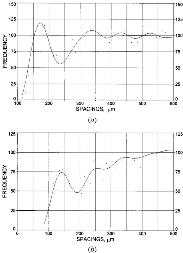
Fig. 3—Typical distribution of nearest and higher-order neighbor spacing (thermal gradient  $G_L = 86$  K/cm): (a) dendritic growth at  $V = 18.4 \mu\text{m/s}$  and (b) cellular growth at  $V = 1.5 \mu\text{m/s}$ .
