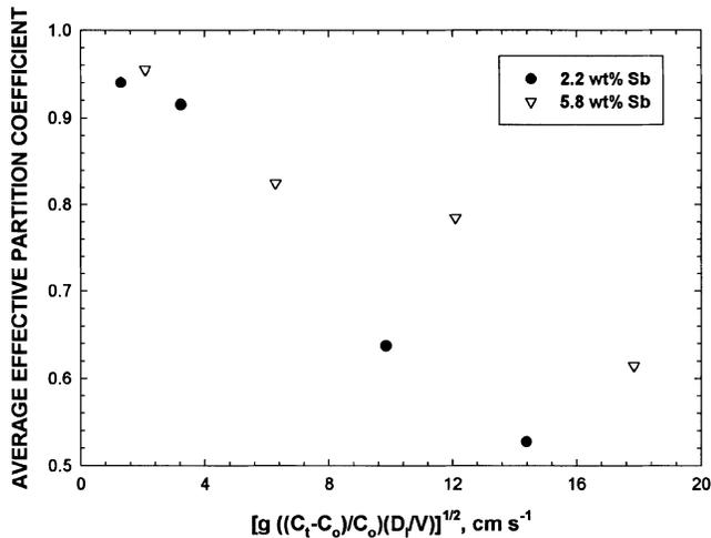
Fig. 6—Correlation between the extent of longitudinal macrosegregation as indicated by the effective partition coefficient and the parameter  $[g(C_t - C_o)D_l/VC_o]^{1/2}$ , which represents the extent of convection caused by the build up of low density solute at the tips of cellular/dendritic arrays during directional solidification of hypoeutectic Pb-Sb alloys.
