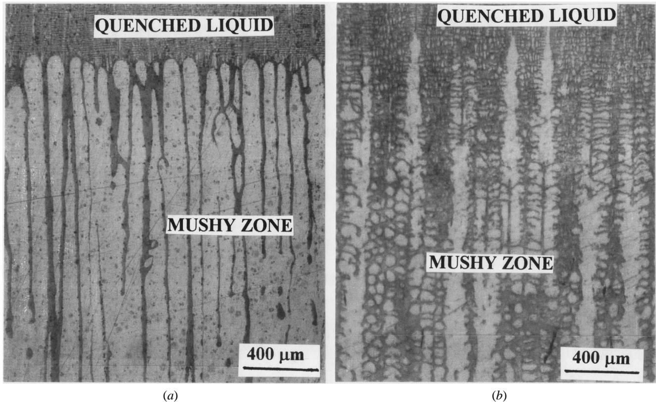
Fig. 1—Typical longitudinal microstructures of directionally solidified Pb-5.8 wt pct Sb alloy near the quenched cellular/dendritic array tips: (a) cellular array ( $V = 0.8 \mu\text{m s}^{-1}$ ) and (b) dendritic array ( $V = 3.0 \mu\text{m s}^{-1}$ ).
