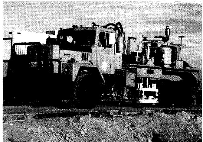
FIG. 5. Rolling Dynamic Deflectometer (RDD)
