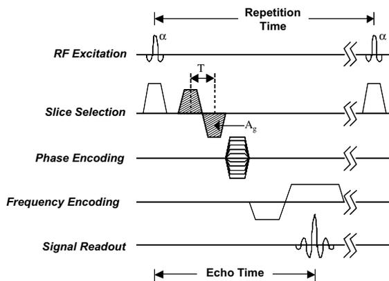
Fig. 1. A simplistic diagram of an unsegmented gradient-echo MR sequence with a bipolar gradient (shaded area) for velocity encoding in the slice selection direction ( $\alpha$ : flip angle,  $A_g$ : bipolar gradient single lobe area,  $T$ : time between the lobe centers in the bipolar gradient).
