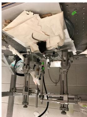
Figure 1: Stereotaxic Apparatus
