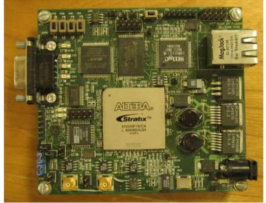
Fig. 3. FPGA-based RCCM.
