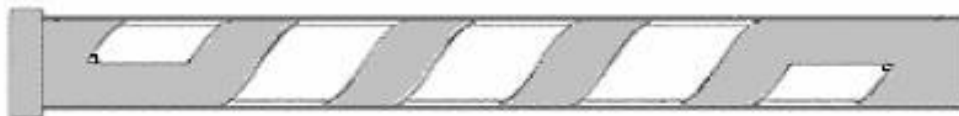
Figure 4.5. Longitudinal section of the 250 \mu\text{m} thick helical channel inserted into the stainless steel cylinder. The inlet and outlet ports are shown as small circles at the ends of the channel.
