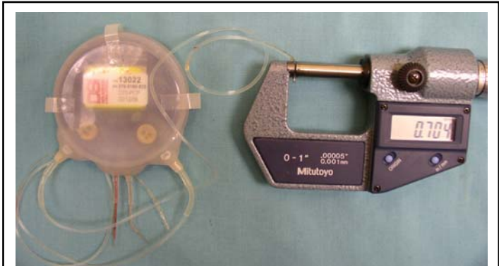
Figure 4.1: The DSI telemetric pressure transducer housing two pressure sensors within the fluid-filled catheters, with one catheter being compressed to a measured displacement to demonstrate the catheter compliancy.
