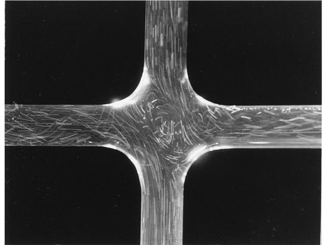
Fig 7. Particle flow visualization of flared design 1 (flaring on all sides with zero offset) model with flow splits: IVC:SVC 60:40 and RPA:LPA 50:50.
