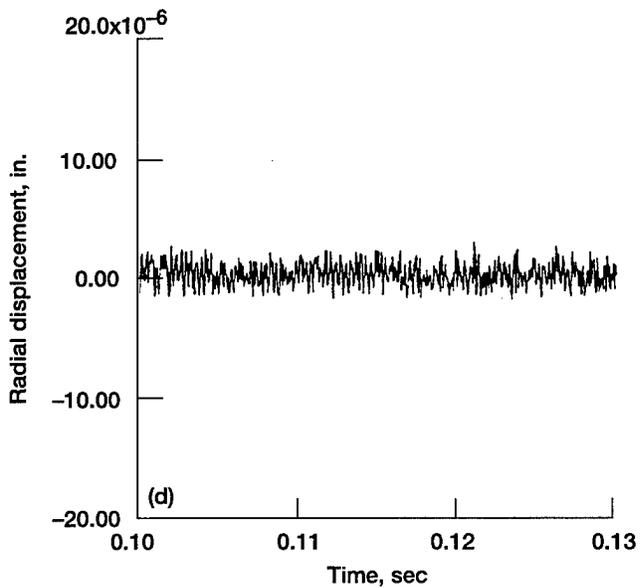
Fig. 8.—Gearshaft radial displacement from mean position for the case of  $0^\circ$  phasing of dual power paths showing vibration levels for all gearshaft supports. (a) Left compound shaft. (b) Right compound shaft. (c) Input pinion shaft. (d) Bull gear shaft.
