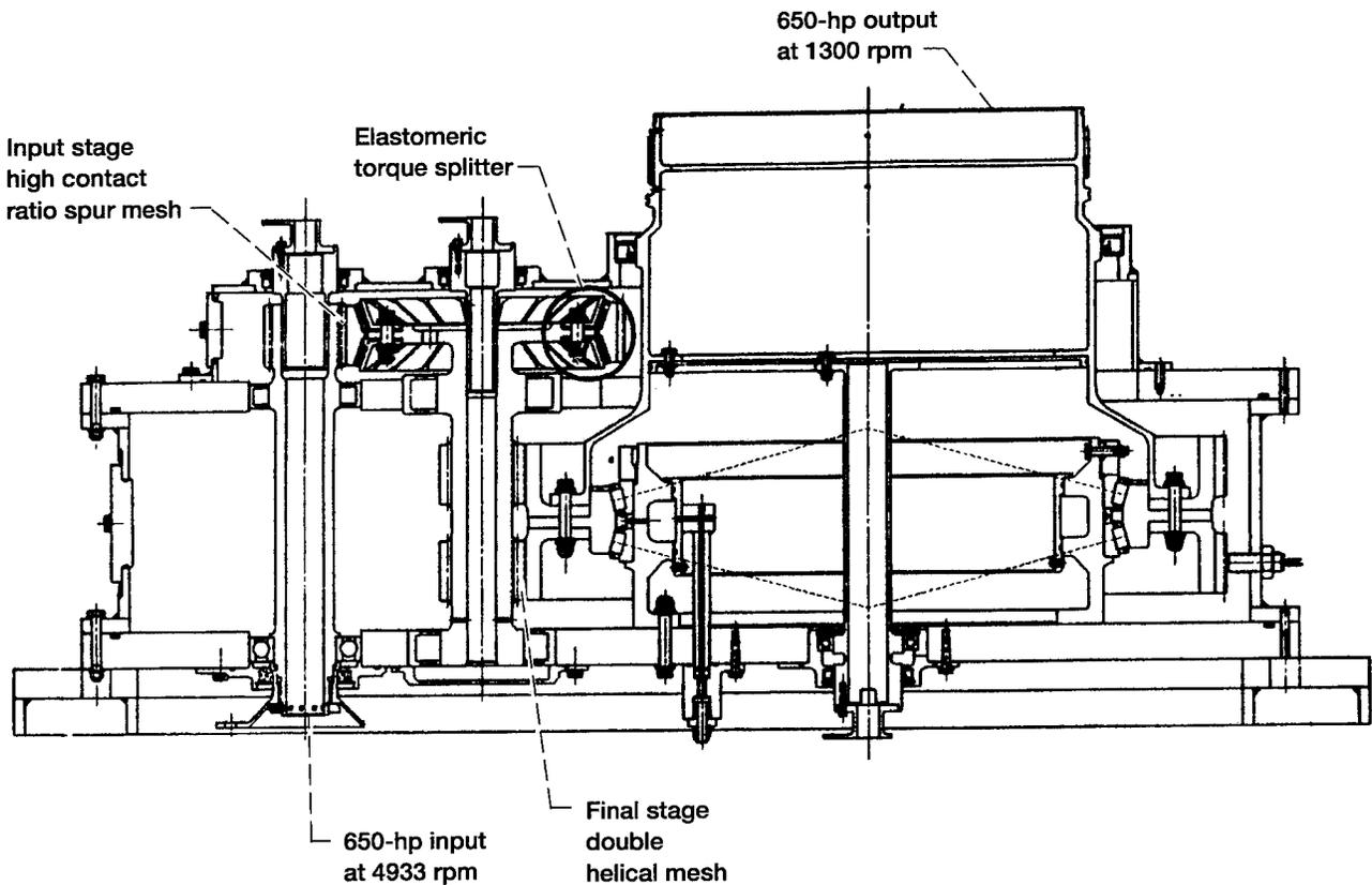
Fig. 1.—Cross-sectional view of the ART split path test gearbox<sup>[8]</sup>.
