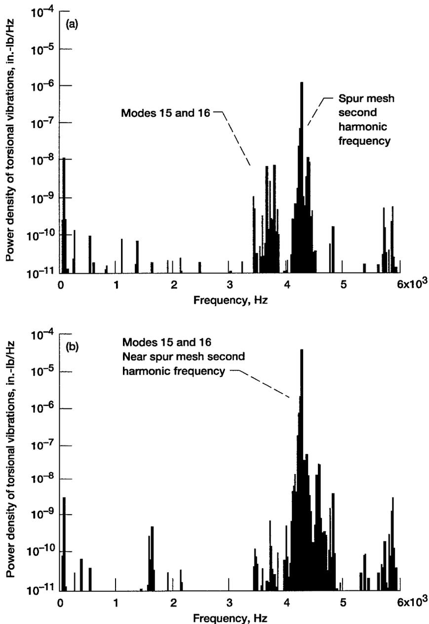
Fig. 16.—Spectrum of power density of shaft torsional vibration energy for right compound shaft at two stiffnesses. (a) Compound shaft stiffness =  $3.0 \times 10^6$  in.-lb/rad. (b) Compound shaft stiffness =  $7.8 \times 10^6$  in.-lb/rad.
