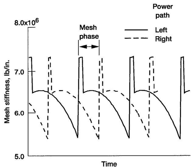
Fig. 4.—Time-varying spur mesh stiffness showing mesh phase.
