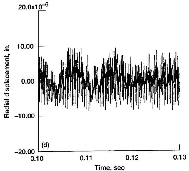
Fig. 9.—Gearshaft radial displacement from mean position for the case of  $90^\circ$  phasing of dual power paths showing large increase in vibration levels for all gearshaft supports. (a) Left compound shaft. (b) Right compound shaft. (c) Input pinion shaft. (d) Bull gear shaft.
