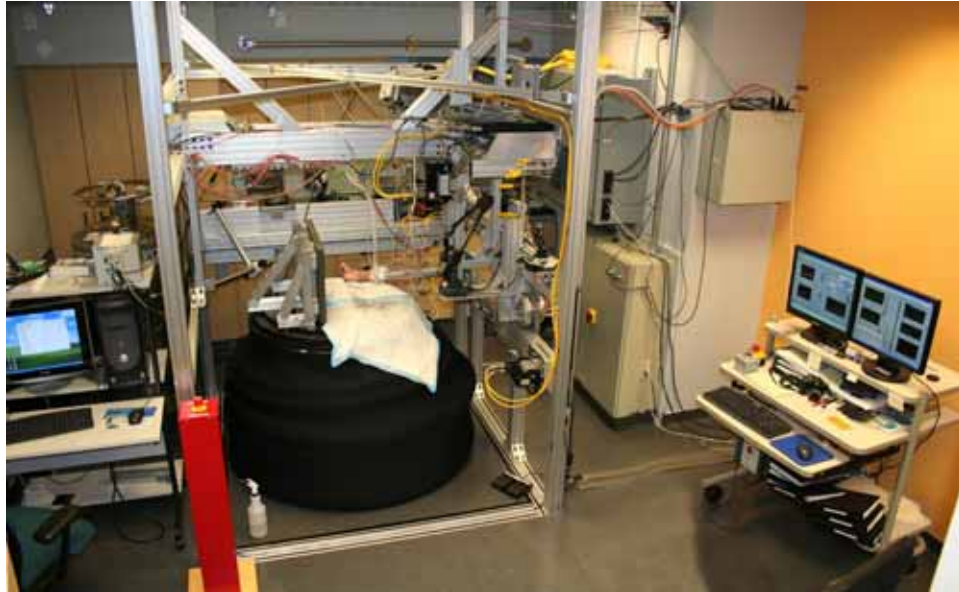
Figure 2.1. The UMS with a horizontally mounted cadaver foot specimen.
