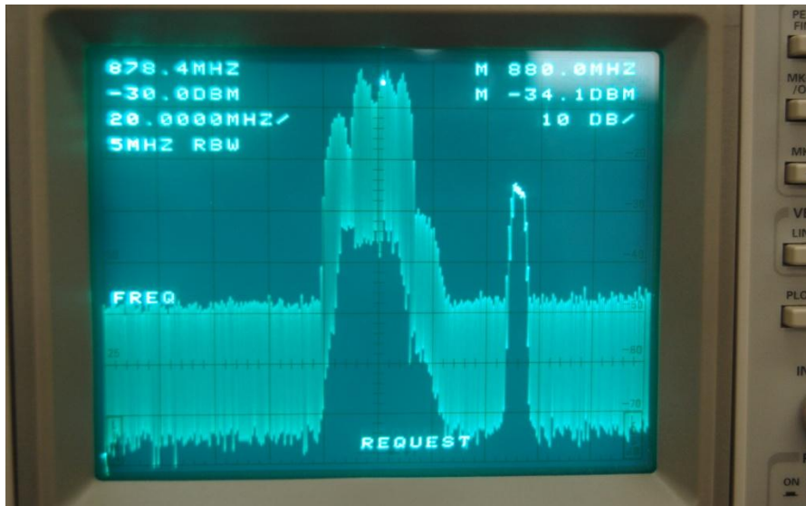
Fig. 3.2: The center frequency of the RF signal emitted by the cell phone used shows a reading of 878 MHz.
