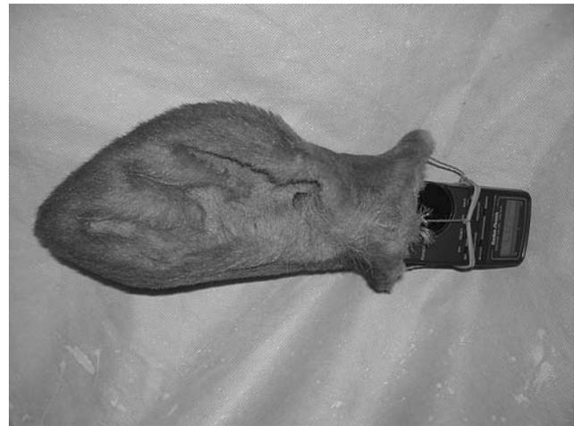
**Fig. 2** Sound meter inserted into the artificial ear
