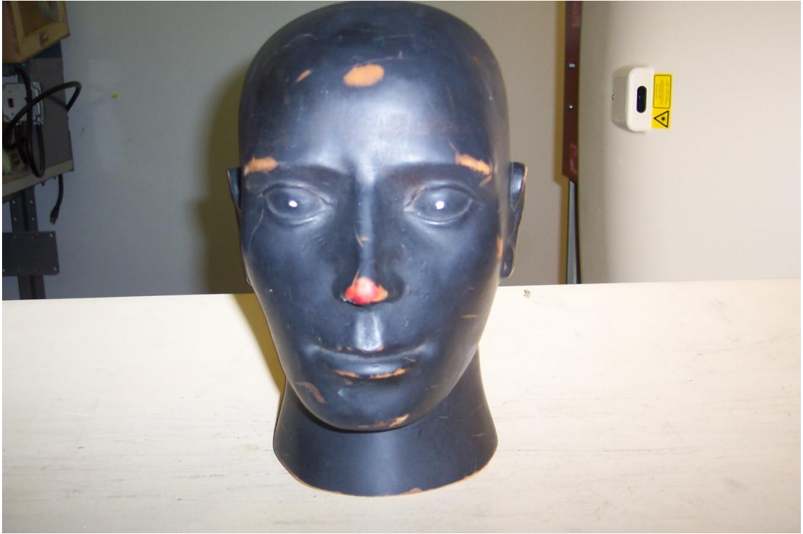
Figure 50: Head Phantom Used for this Research
