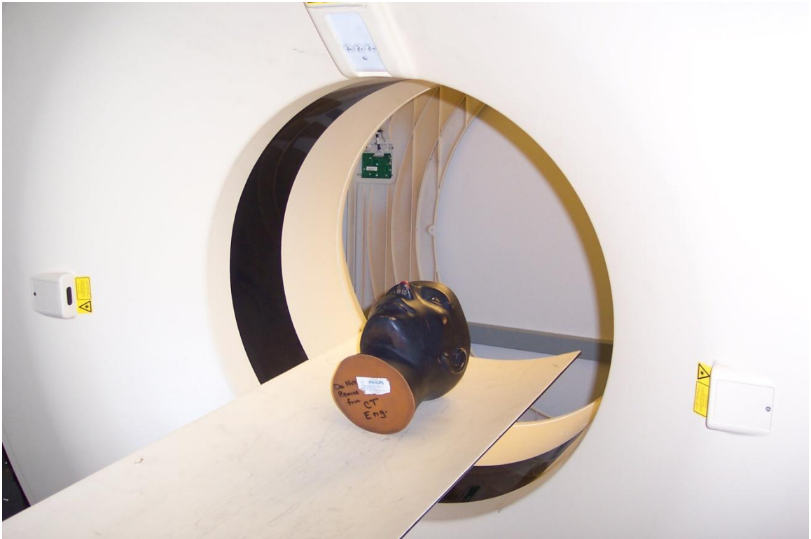
Figure 49: Close-up View of Head Phantom Placed for Scanning
