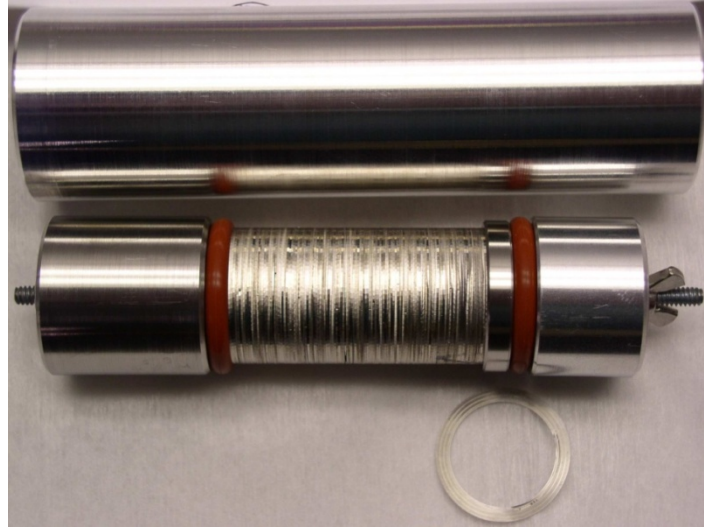
Figure 18.—The regenerator in its fixture after arrival at Sunpower.
