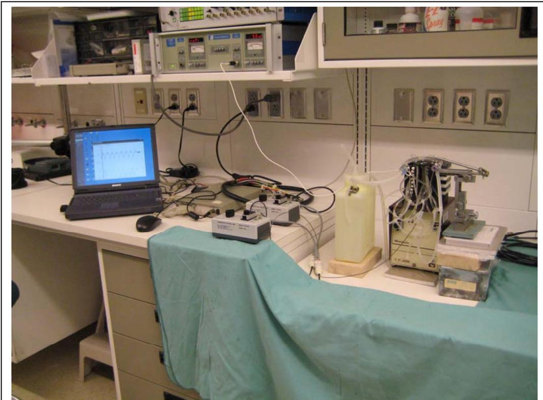
Figure 14: Photograph of the Mock II Circulatory Circuit.
