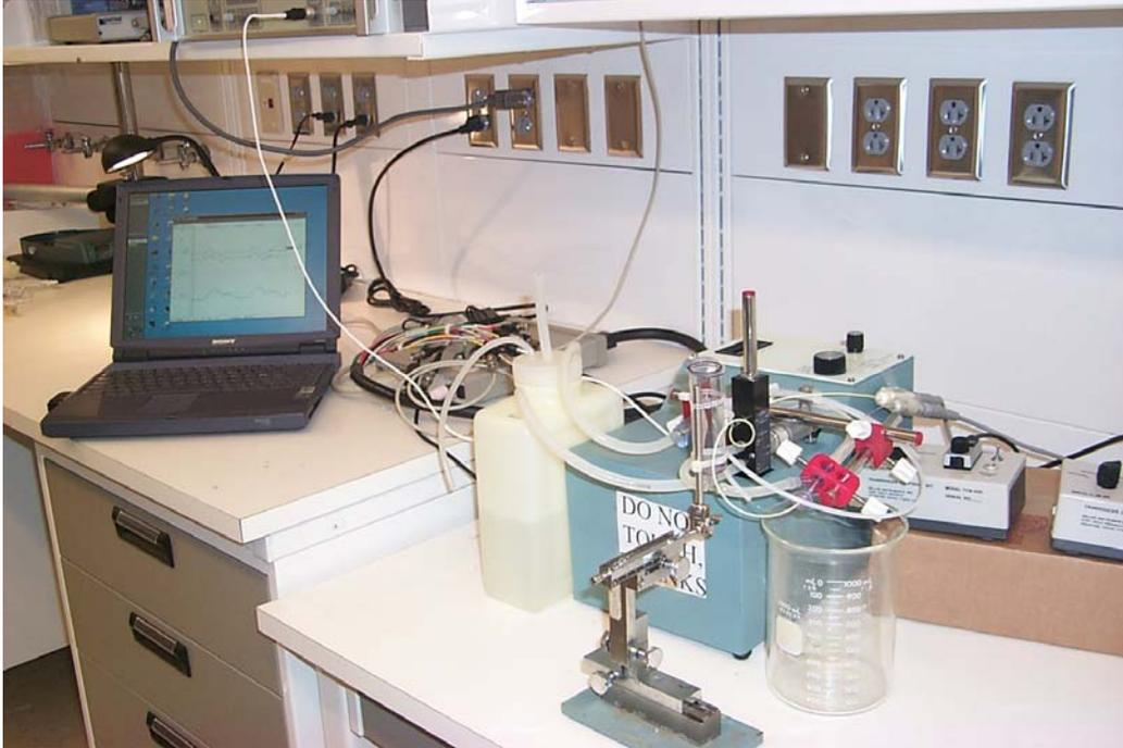
Figure 13: Photograph of the Mock I Circulatory Circuit.
