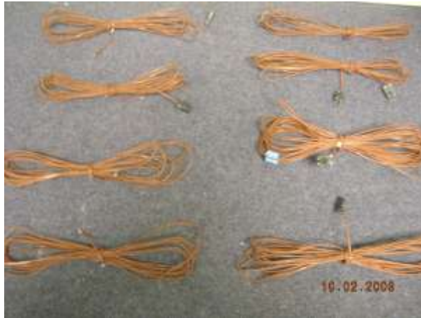
Figure 8: Thermocouples used in the experiment. Courtesy: [HMI Industries]
