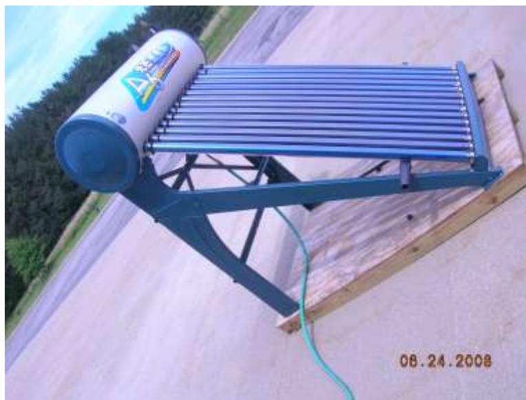
Figure 15: Closed Loop Static Testing.
