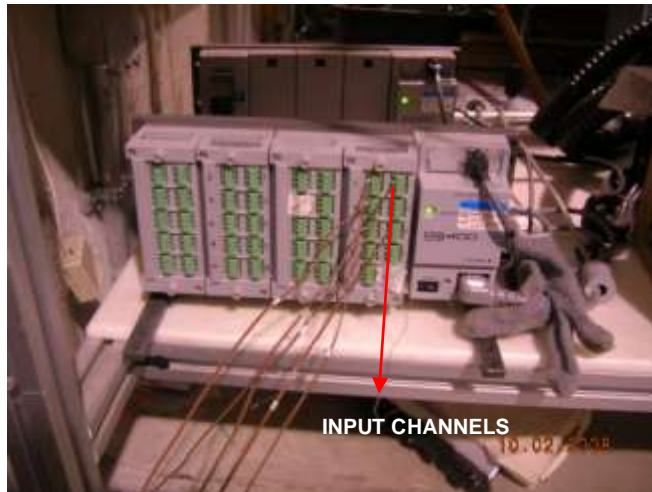
Figure 10 : Input module of the DARWIN system. Courtesy: [HMI Industries]
