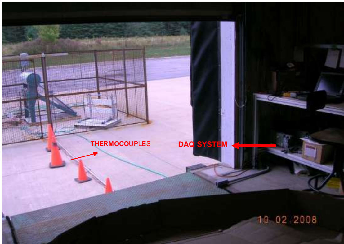
Figure 21: Interface between Solar Water Heater and DAQ System.
