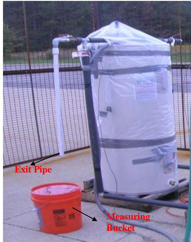
Figure 18: Recover Rate Test of HWT. Courtesy: [HMI Industries]
