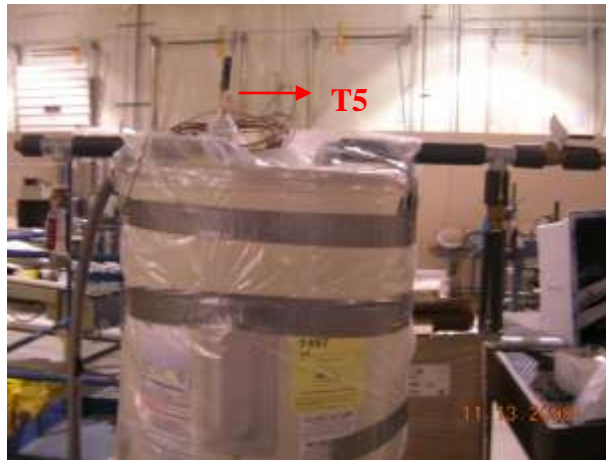
Figure 17: Probe thermocouple on Hot Water Tank.
