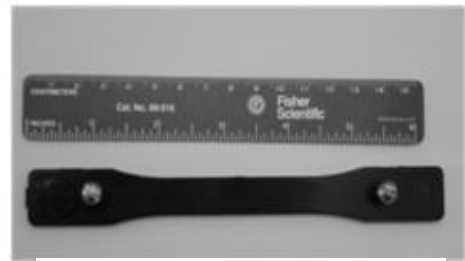
Figure 4.5: Tensile Bar with Two Brass Screws apart
