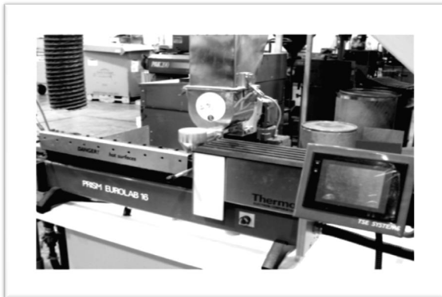
Figure 4.3: Extruder Used for Compounding Composites
