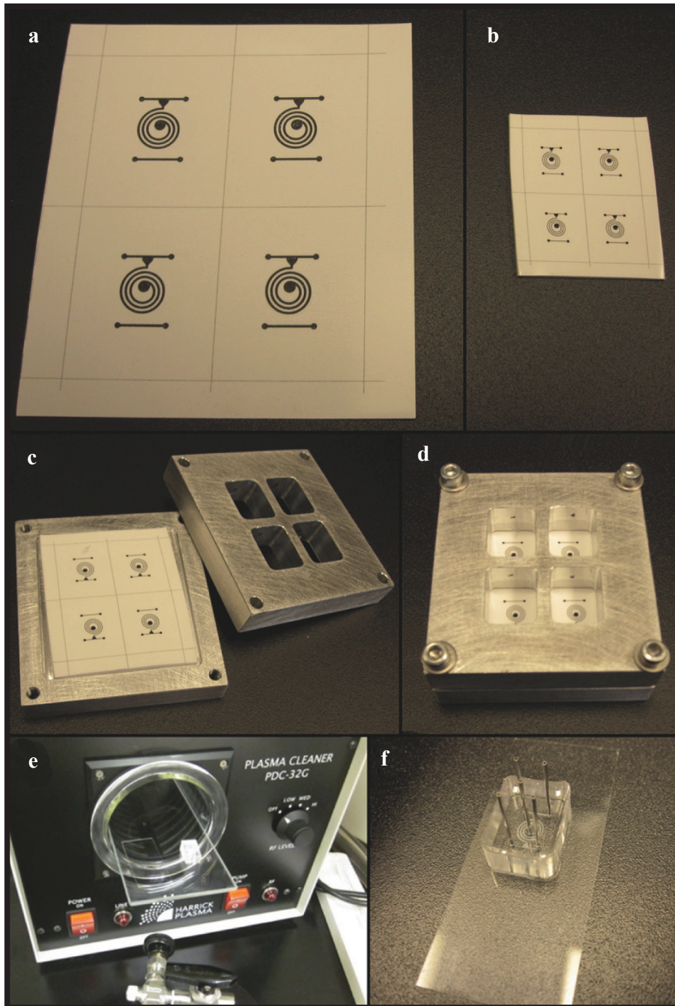
Figure 6: Overview of shrinky dink chip fabrication. a) Pre-shrunk pattern. b) Shrunk pattern. c) Pattern in holder. d) PDMS curing. e) Chip and coverslip being placed in plasma cleaner. f) Chip bonded to glass coverslip.
