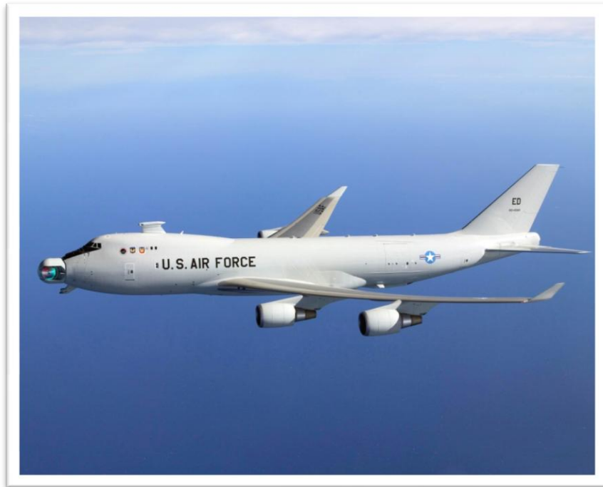
Figure 29: Boeing ABL with Laser Turret [38]
