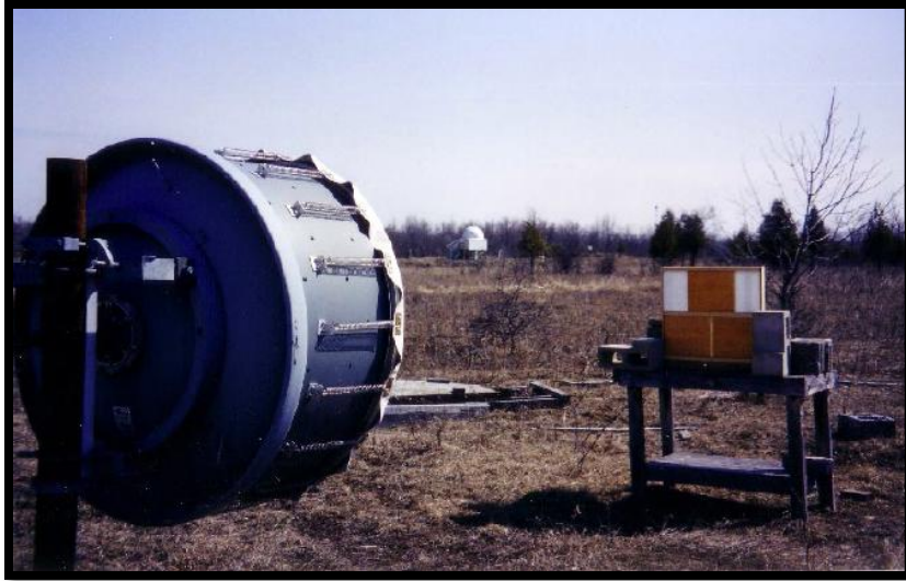
Figure 8: Microwave Transmitter (left) and Rectenna [18]
