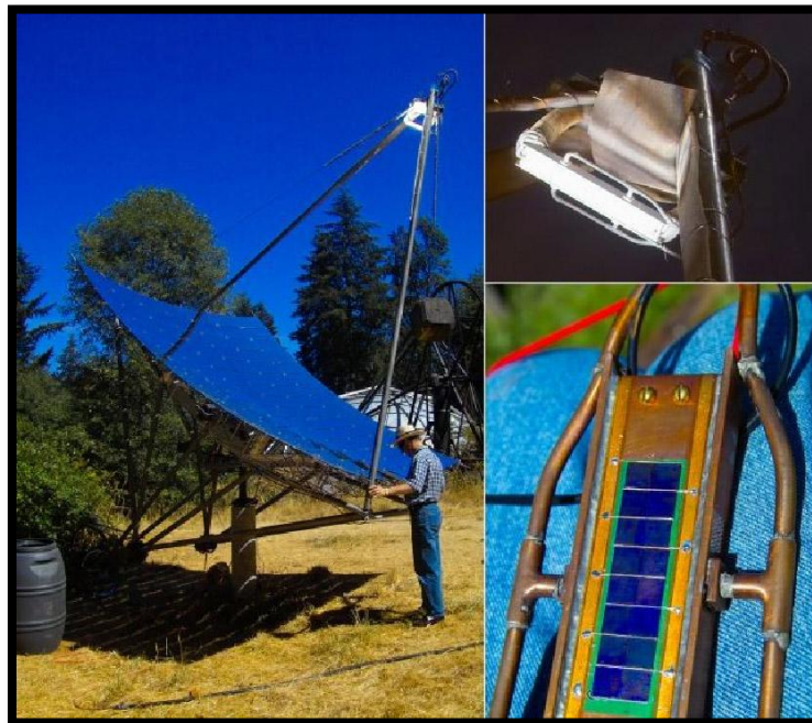
Figure 21: VMJ Cells in a 9 kW Solar Concentrator
