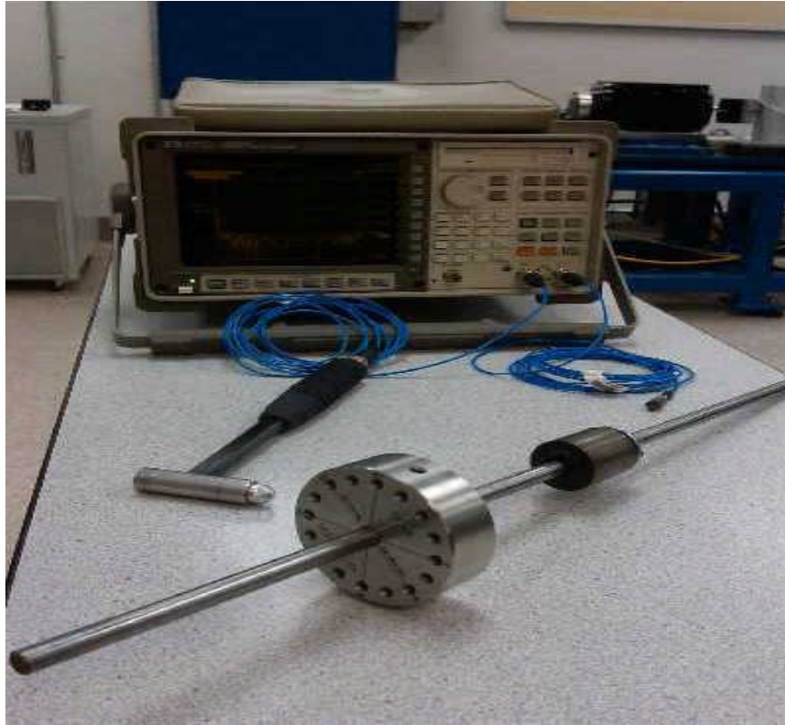
Figure 4.1 Hewlett Packard 35670A dynamic signal analyzer, impulse hammer, accelerometer and assembled rotor removed from bearings.
