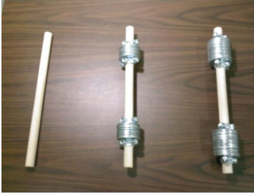
Figure 7. The weights, 0 kg, 1 kg, and 1.5 kg (from left to right). The 0 kg weight consisted of a wooden dowel and the 1 kg and 1.5 kg weights consisted of metal washers attached to a dowel.
