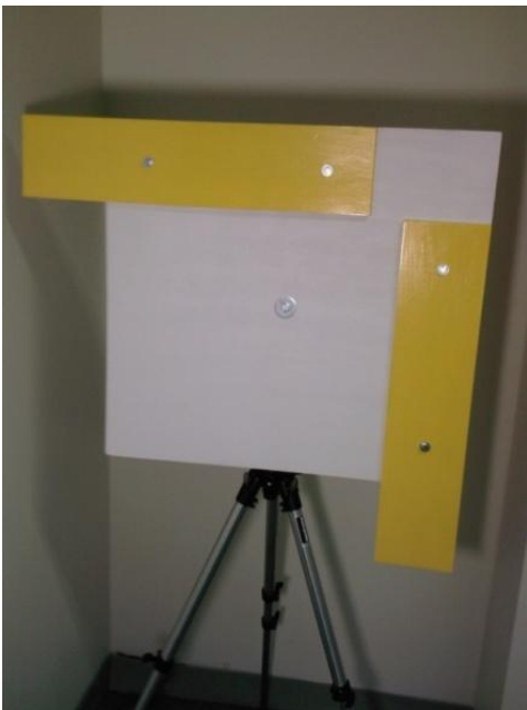
Figure 6. The target board consisted of two yellow targets and a white board mounted on an adjustable tripod.
