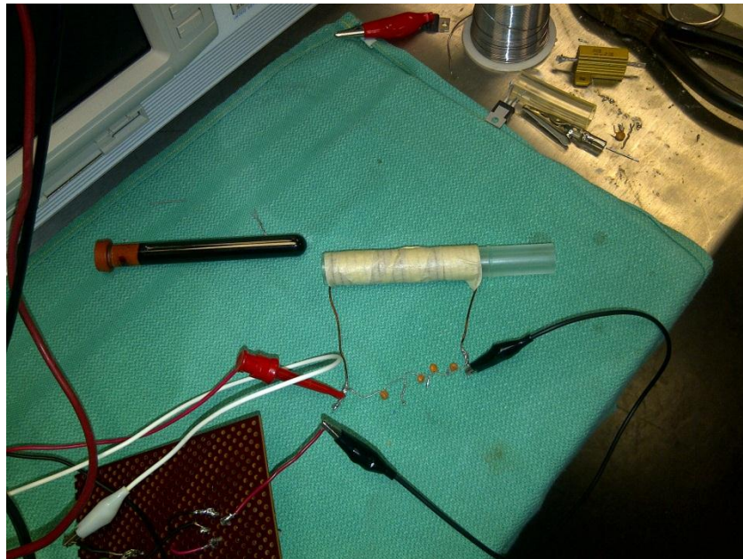
Figure 29 -- The picture of the 1 \mu\text{H} air core coil and the experiment tubing which is filled with ferrofluid
