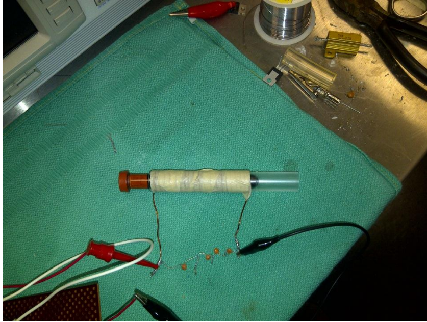
Figure 30 -- The picture of the ferfluid tubing while inserted into the air core coil
