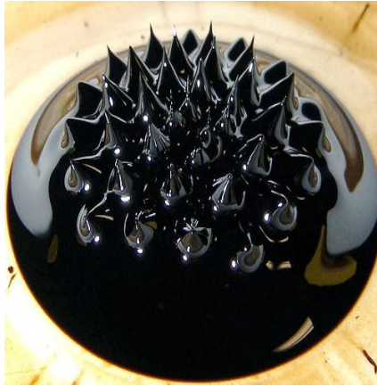
Figure 5 -- illustrates that the movement of the ferrofluid magnetic particle when an external magnetic field is applied
