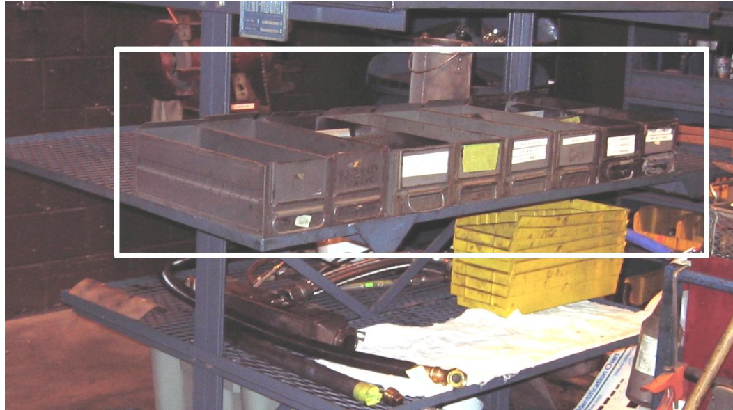
Figure 13: Special bolts bins ( poka-yoke device)
