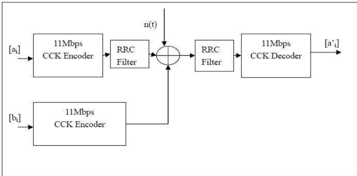
Figure 17: 802.11b 11Mbps with another 11Mbps interferer system model
