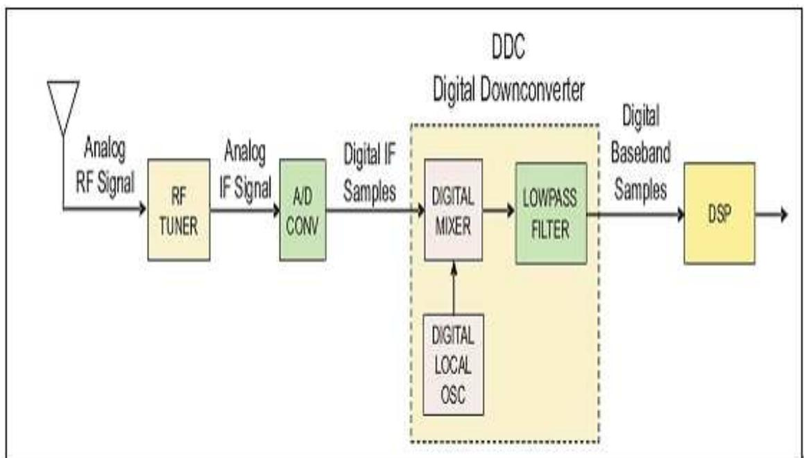
Figure 9: SDR receiver block diagram [12]
