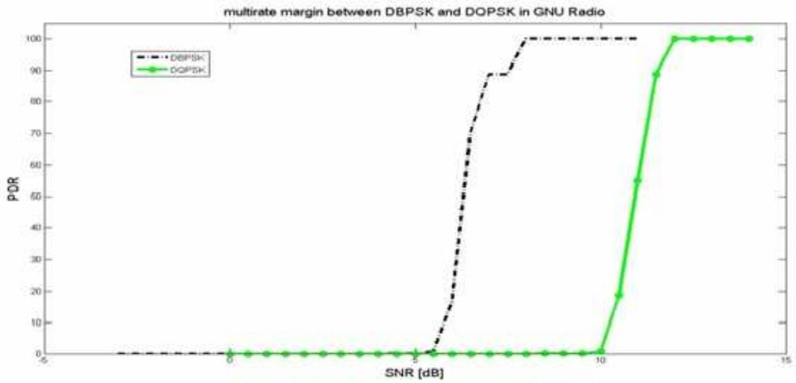
Figure 29: PDR Simulation Result for DBPSK and DQPSK without RS code
