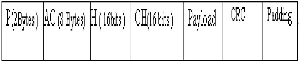
Figure 32: Transmitted frame (padding code is to add some padding at the end of the packet to fit the needs of USRP)
