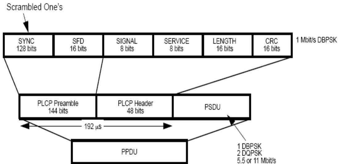
Figure 5: Long PLCP PDU format [1]
