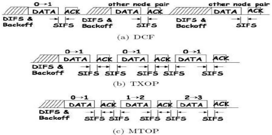
Figure 38: DCF, TXOP and MTOP packet transmission protocol[41]
