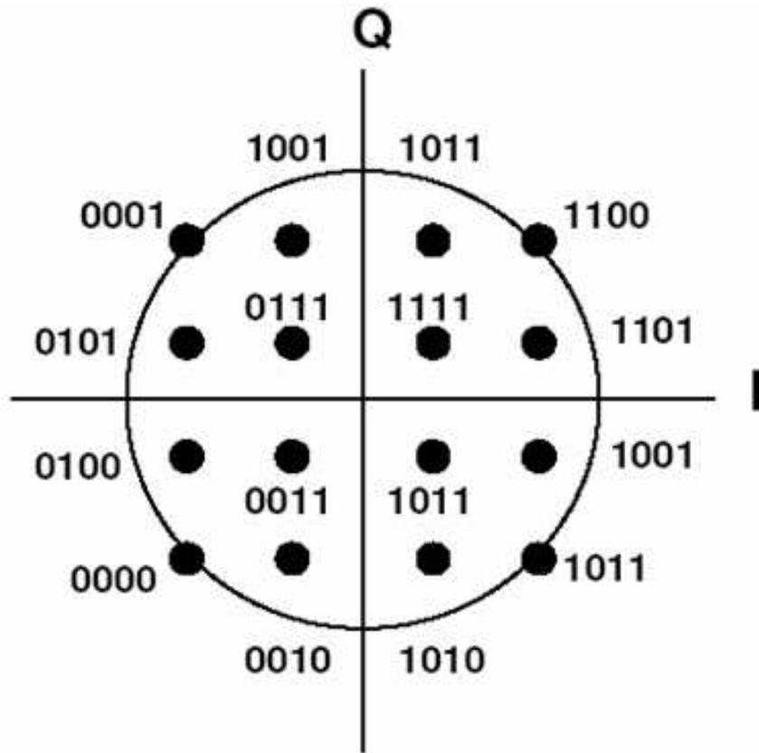
Figure 4: Constellation Picture for 16QAM [4]
