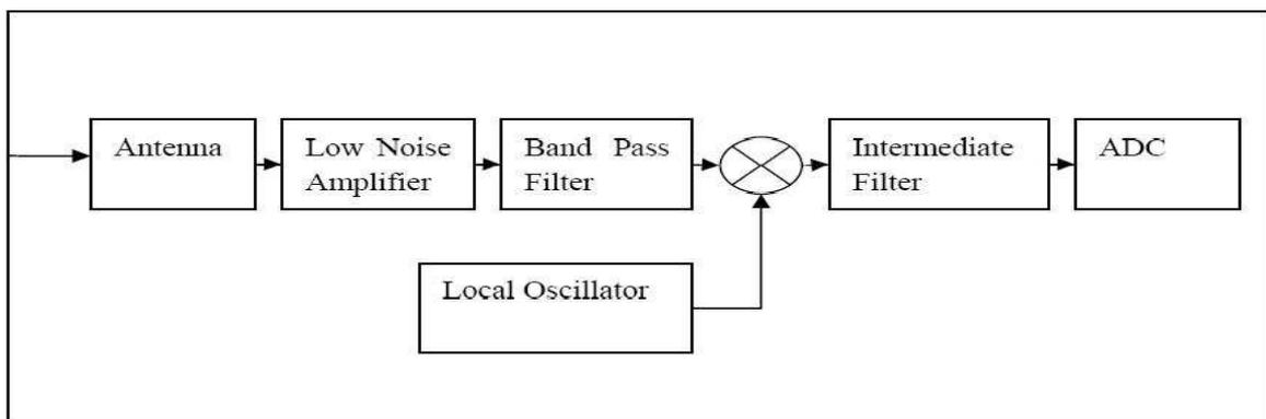
Figure 22: A typical structure of RF front end
