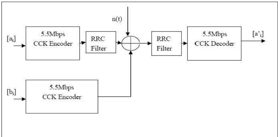
Figure 19: 802.11b 5.5Mbps with another 5.5Mbps interferer system model
