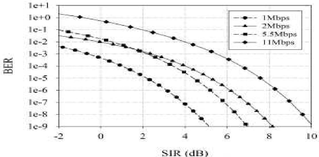
Figure 11: BER versus SIR in 802.11b[30]
