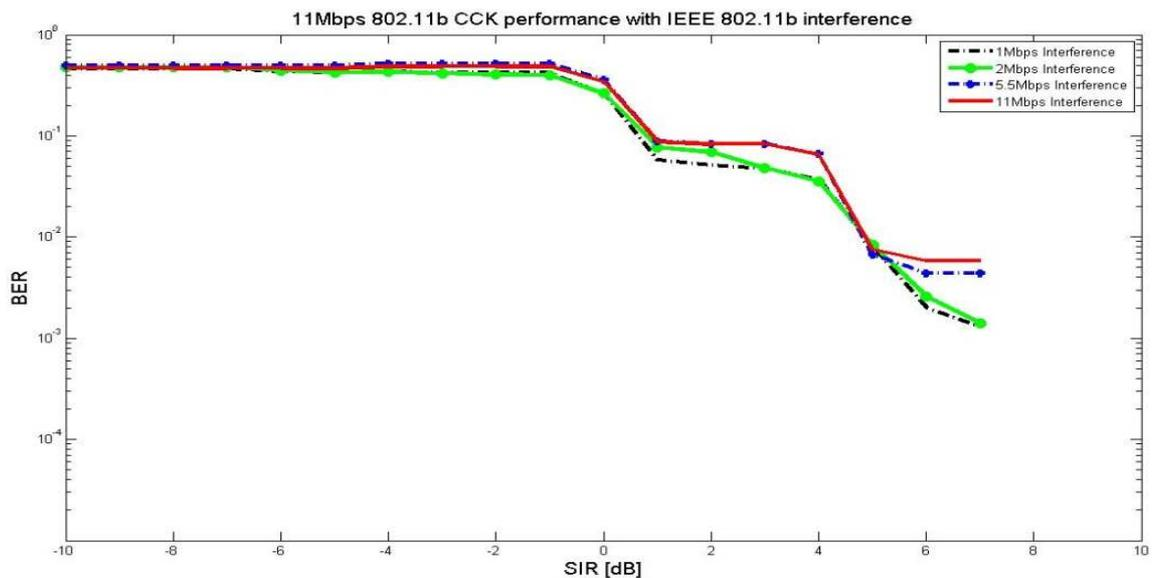
Figure 18: 11Mbps 802.11b performance with IEEE 802.11b interference. AWGN channel. SNR = 35dB
