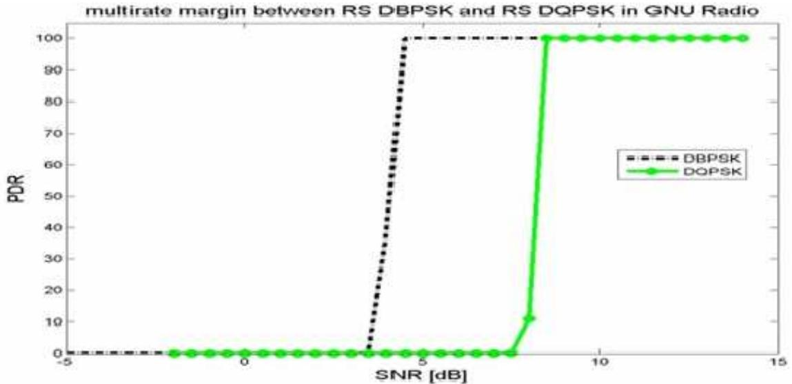
Figure 31: PDR Simulation Result for DBPSK and DQPSK with RS code
