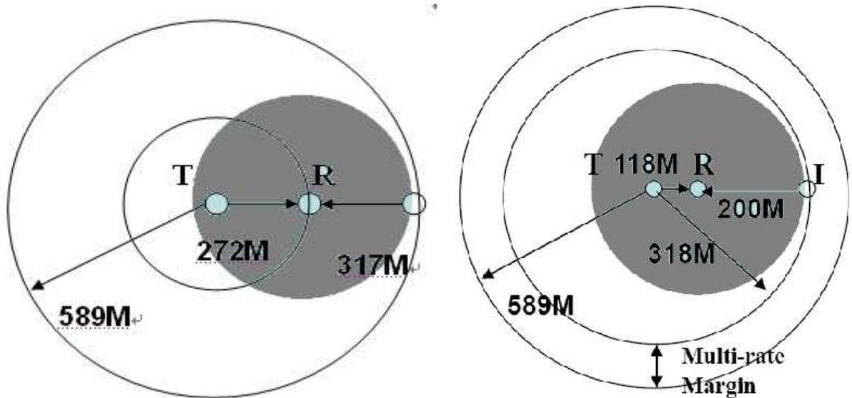
Figure 12: Interference and the required defer range (the required defer range in the right diagram is 271 meters smaller than that in the left but as the same defer range is used in the network, the extra space at 11Mbps mode would be utilized in MTOP).
