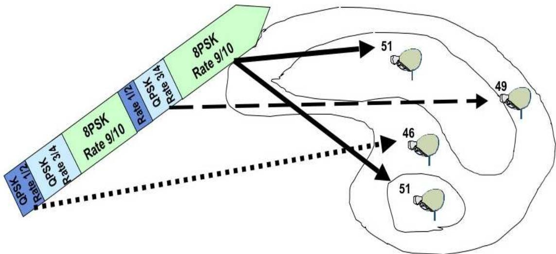
Figure 1: Sample satellite footprint with downlink EIRP values[40]
