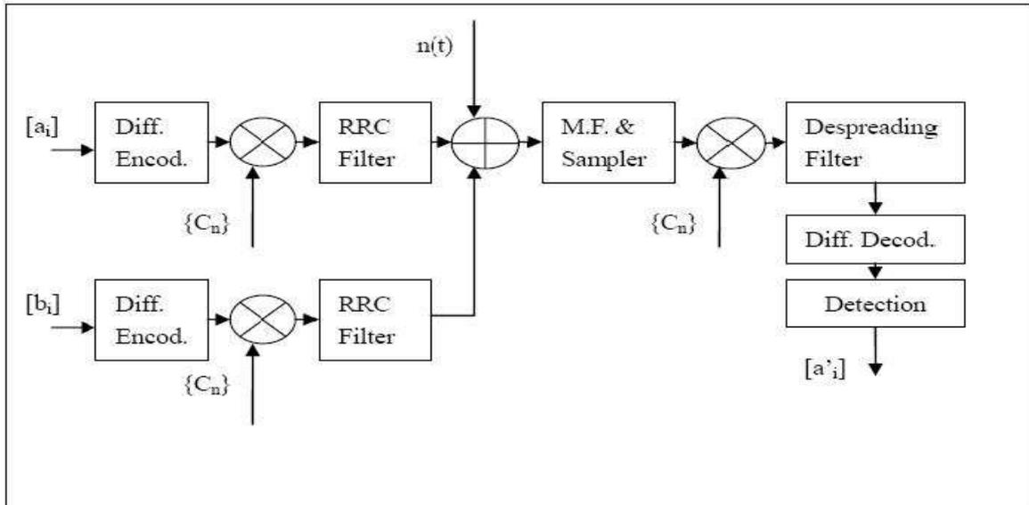
Figure 13: 802.11b DSSS 1Mbps with another 1Mbps interferer system model
