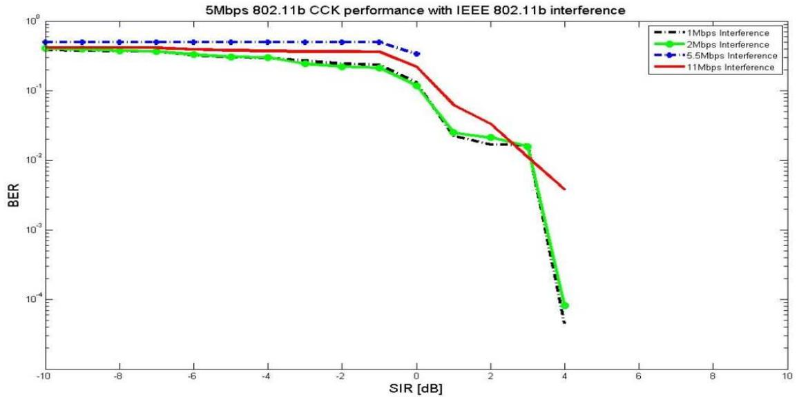
Figure 20: 5.5Mbps 802.11b performance with IEEE 802.11b interference. AWGN channel. SNR = 35dB
