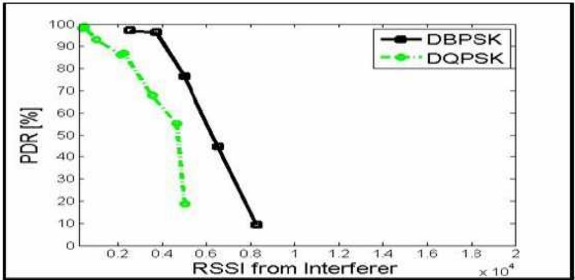
Figure 35: PDR versus RSSI from Interference
