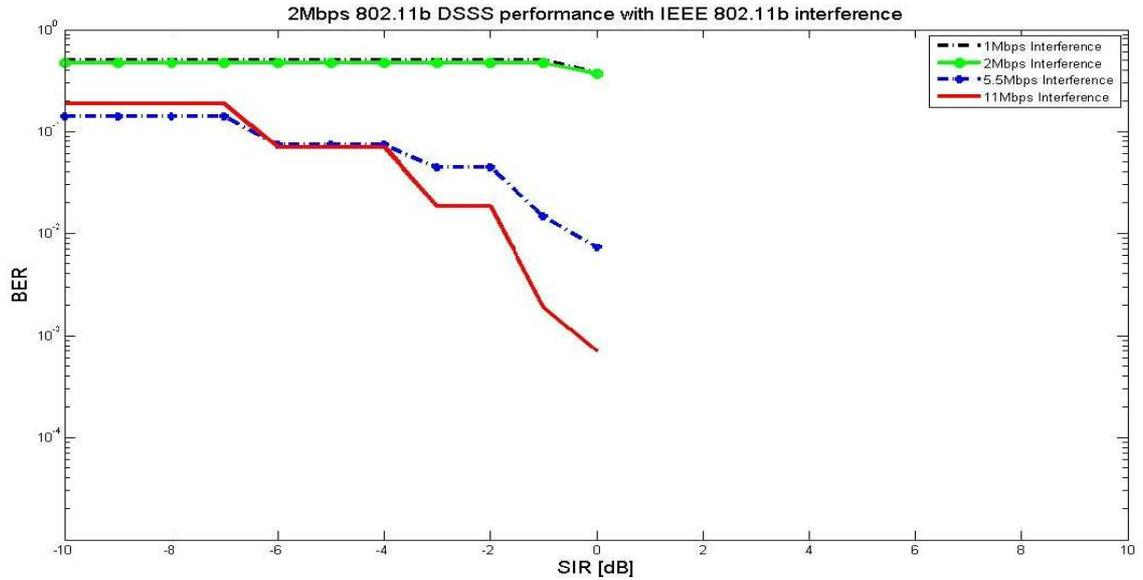
Figure 16: 2Mbps 802.11b performance with IEEE 802.11b interference. AWGN channel. SNR = 35dB
