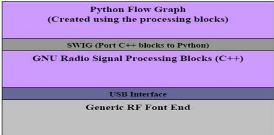
Figure 21: Block Diagram of GNU Radio Components[14]
