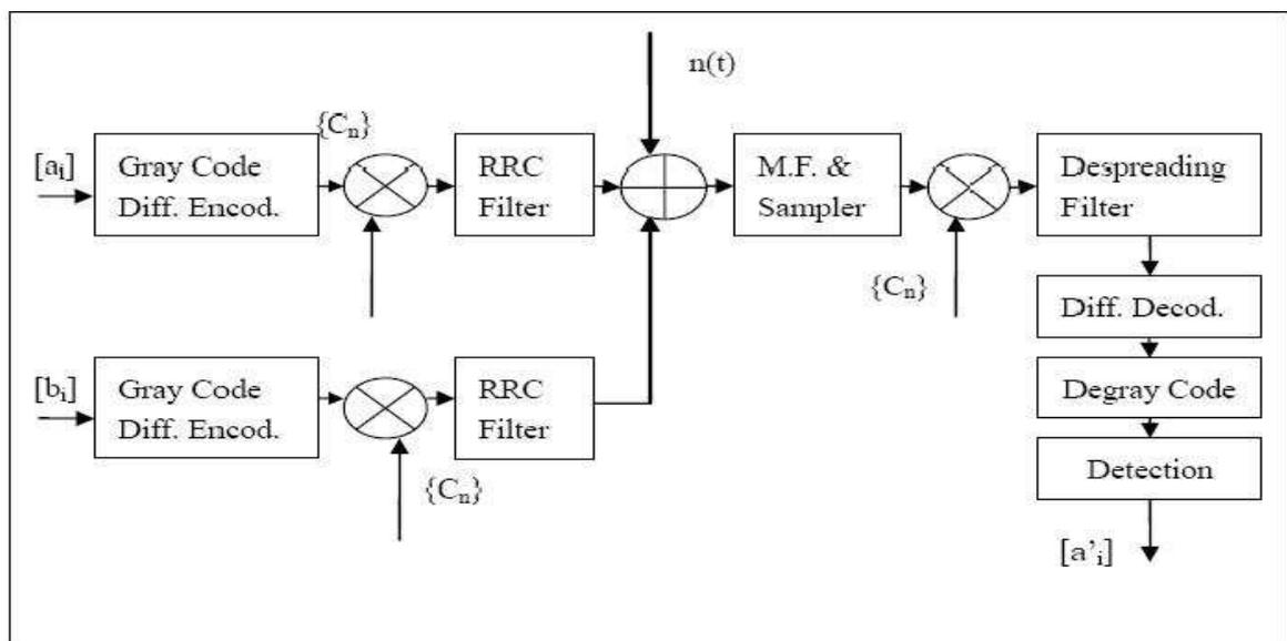
Figure 15: 802.11b DSSS 2Mbps with another 2Mbps interferer system model
