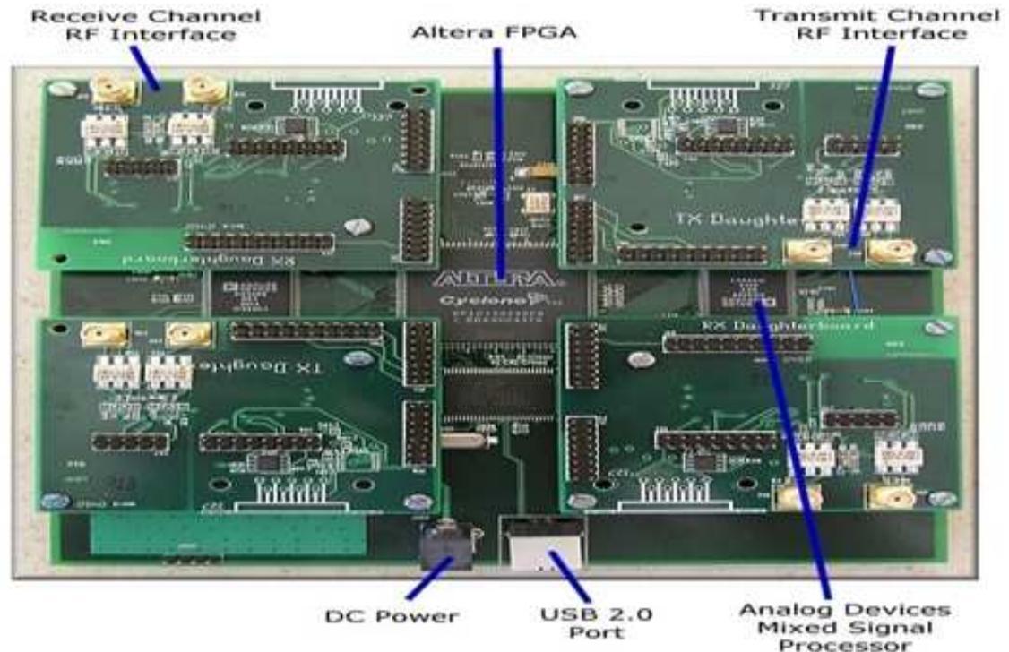
Figure 23: USRP Board (One USRP motherboard can support up to 4 daughterboards and there are an FPGA and two AD/DA converters on one motherboard)
