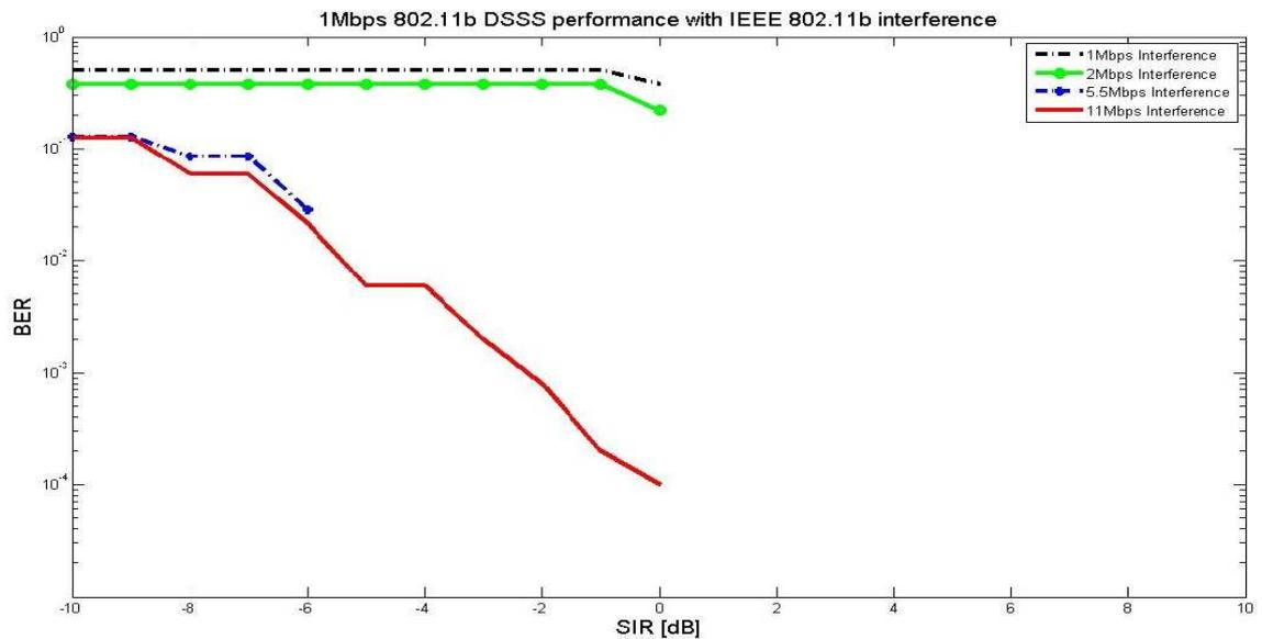
Figure 14: 1Mbps 802.11b performance with IEEE 802.11b interference. AWGN channel. SNR = 35dB
