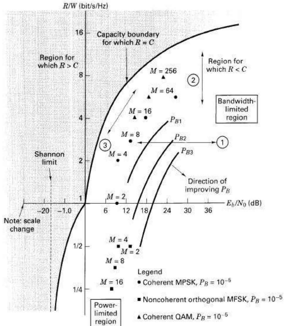
Figure 2: Bandwidth and power efficiency plan [4]
