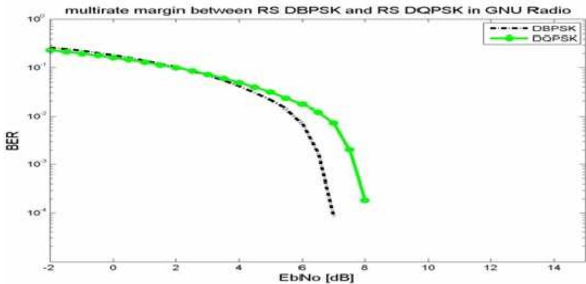
Figure 30: BER Simulation Result for DBPSK and DQPSK with RS code
