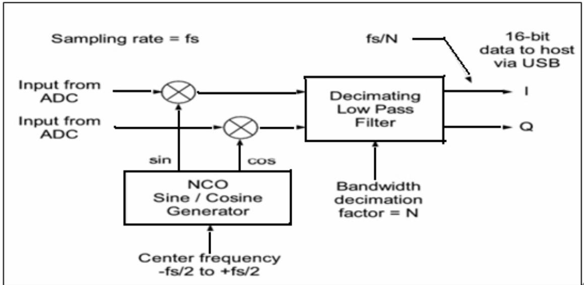
Figure 24: Block Diagram of the Functional Components of FPGA[17]
