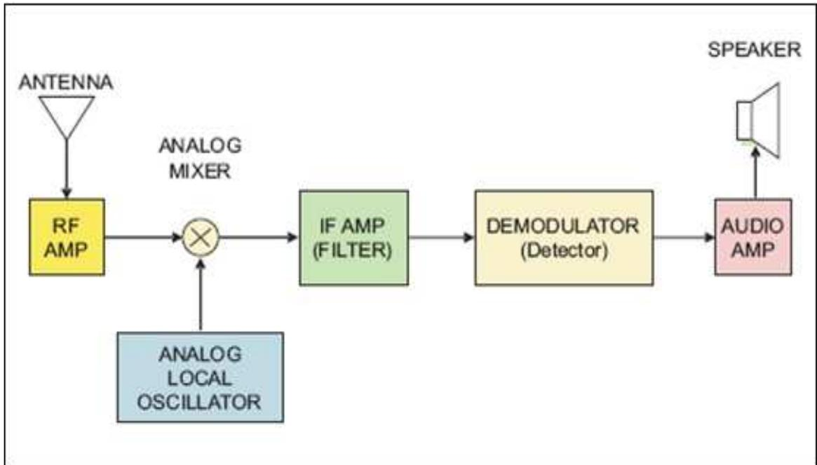
Figure 8: analog radio receiver block diagram[12]
