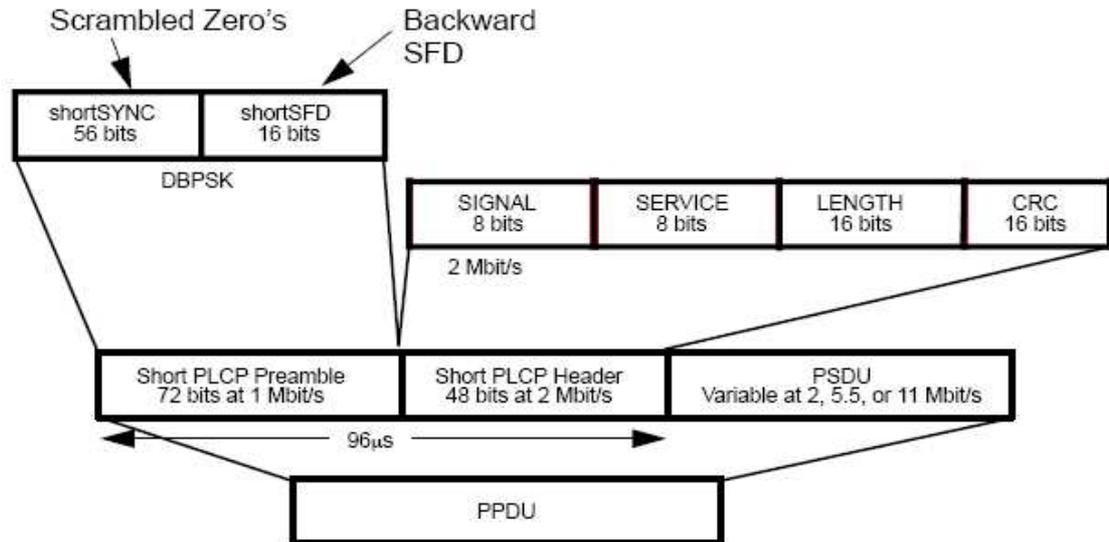
Figure 6: Short PLCP PDU format [1]
