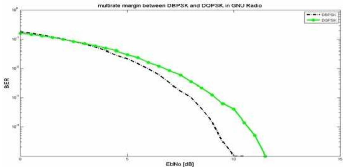
Figure 28: BER Simulation Result for DBPSK and DQPSK without RS code
