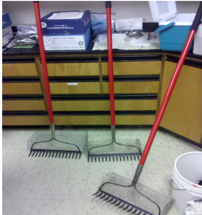
Figure 4. Mussel rakes made from standard bow rakes bought at a consumer hardware store. The basket of the rake was made from 1 cm squared galvanized steel mesh which was wrapped to form a basket. Side panels for the basket portion were cut out using metal shears and all parts were assembled to the rake using 16 gauge steel wire.
