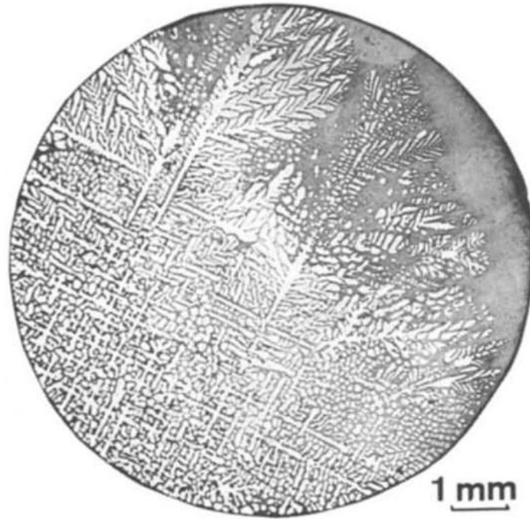
Figure 5: Image of transverse slice of an Al-26.5 wt% Cu copper alloy, grown with 30 \text{ K cm}^{-1} thermal gradient at 4.2 \text{ } \mu\text{m s}^{-1} [12]. This depicts an example of transverse phase macrosegregation.
