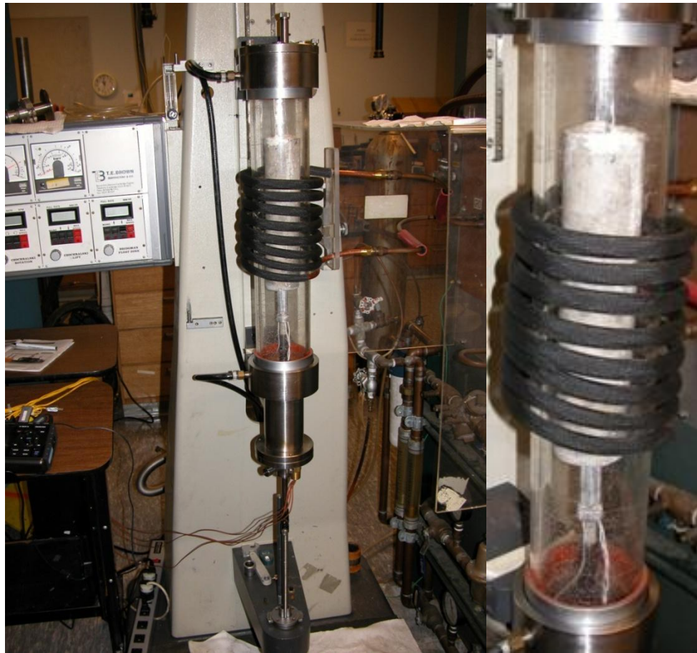
Figure 7: Images of Bridgman-technique furnace assembly for directional solidification
