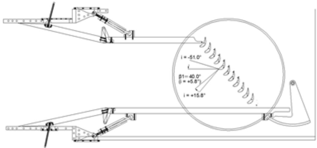
**Figure 1. Cascade Test Section with Blade Geometry.**
