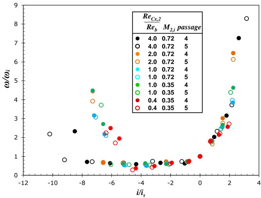
Figure 34. Midspan Loss Bucket on Ainley-Mathieson Scaling.
