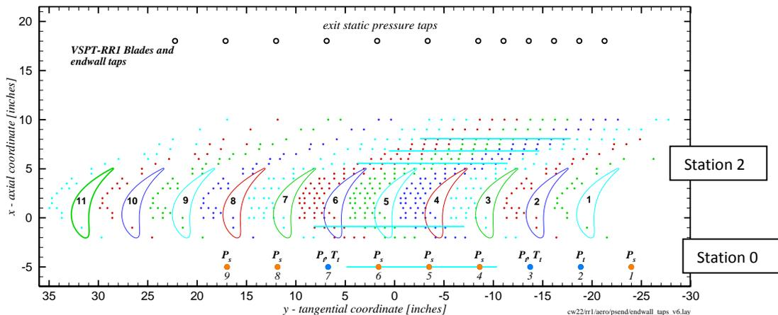
**Figure 8. Endwall Instrumentation Configuration.**
