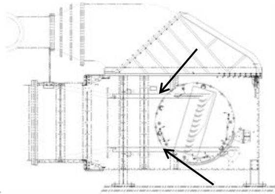
**Figure 4. Facility After Modifications. Arrows indicate flow boards.**
