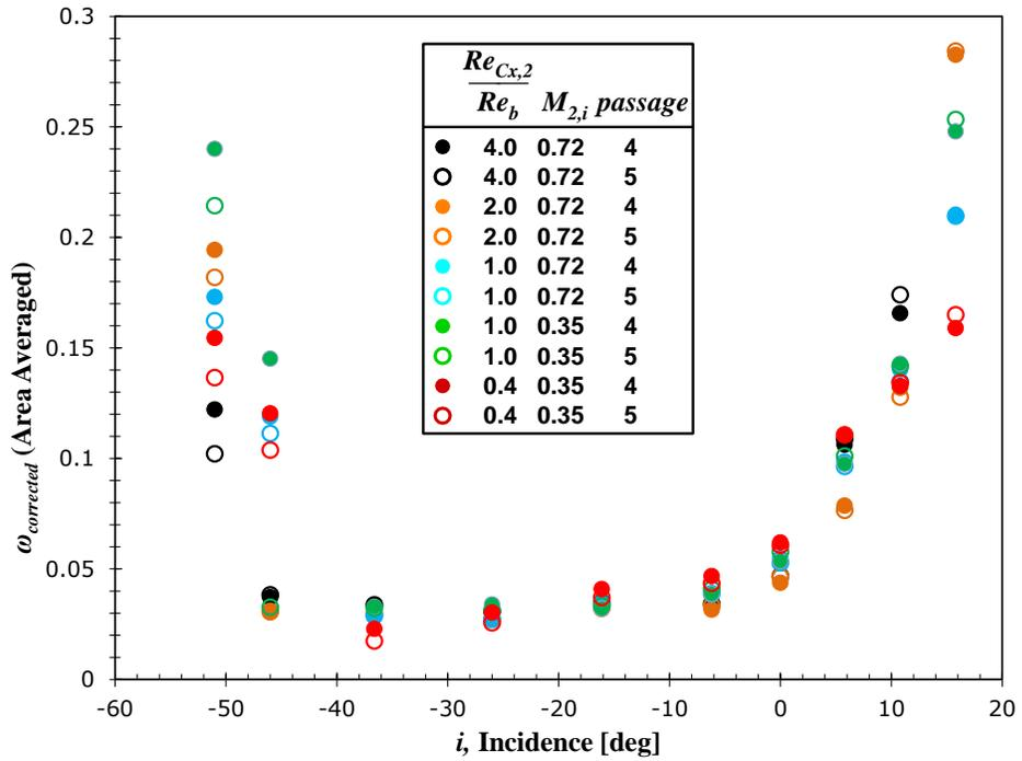
Figure 33.  $Re^{-0.5}$  Scaled Midspan Loss vs. Incidence.
