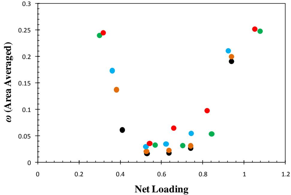
**Figure 35. Midspan Loss vs. Net blade Loading.**
