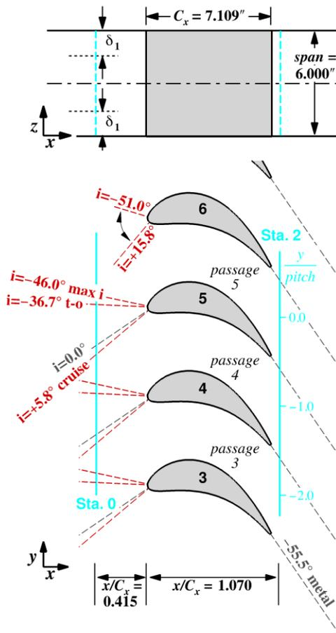
Figure 6. Blade Geometry and Survey Plane Locations.
