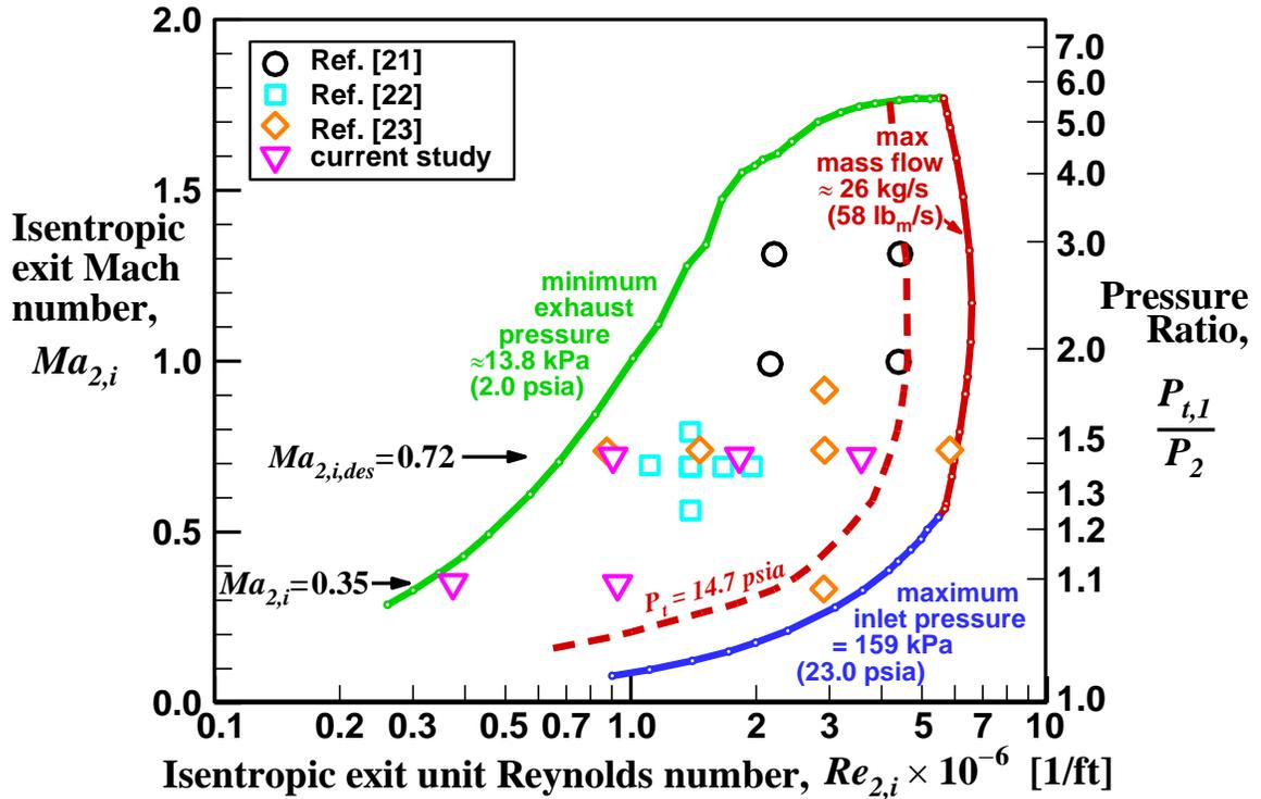
Figure 2. Operating Envelope of NASA Transonic Turbine Cascade.
