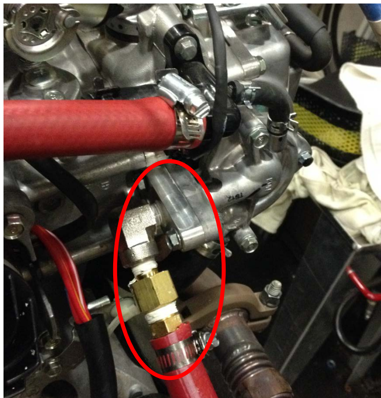
Figure 15 Thermostat Deletion Plate Installed on Engine
