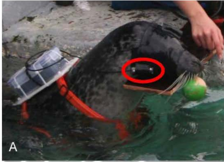
Figure 2: Experimental setup of wake tracking by blindfolded seal. Camera for observing whisker vibration indicated in red [1]
