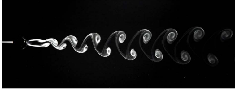
Figure 3: Visualization of a vortex street past a cylinder [21]
