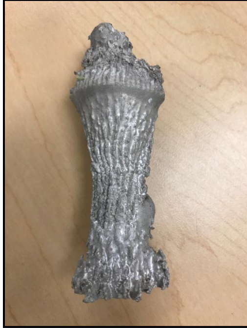
Figure 17: Magnesium billet processed using Electromagnetic Induction
