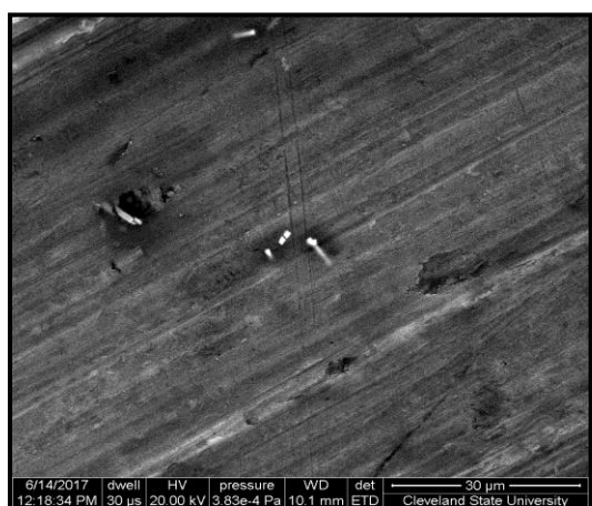
Figure 30: Embedded MWCNTs in Magnesium matrix
