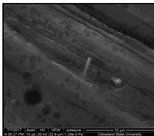
Figure 29: Debris of nanotubes and copper examined with SEM.
