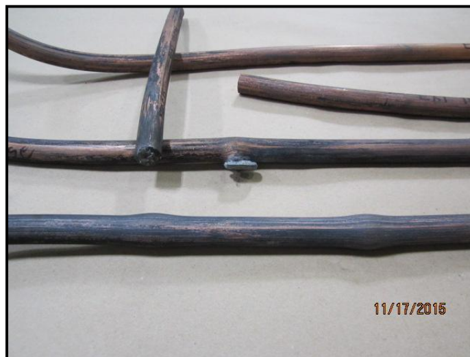
Figure 18: Exploded Cu-Mg/MWCNT composite rod.
