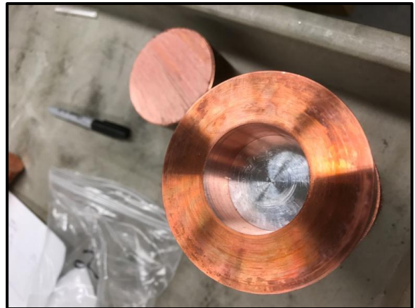
Figure 27: Mg/MWCNT composite embedded in Copper Billet
