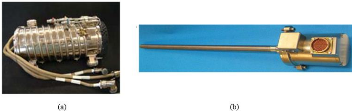
Figure 6 (a) ESA_MSL Low Gradient Furnace (LGF) used for the directional solidification and (b) Sample Cartridge Assembly (SCA), in which a sample for a directional solidification experiment on the ISS is contained 33
