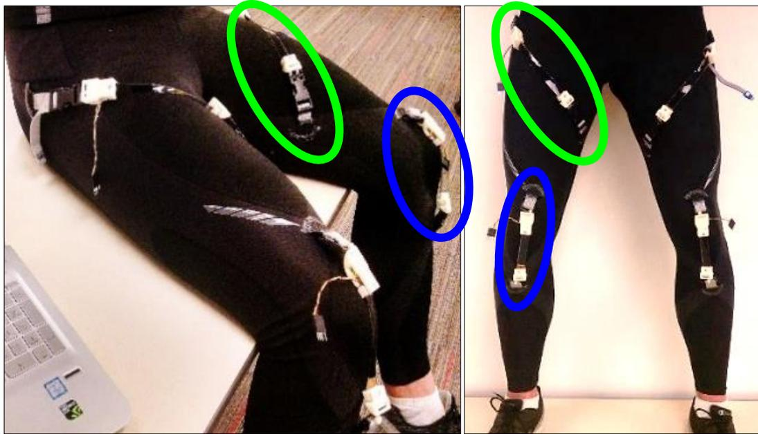
**Figure 11.** The resulting system of flexion (blue) and rotation (green) sensors integrated into compression pants.
