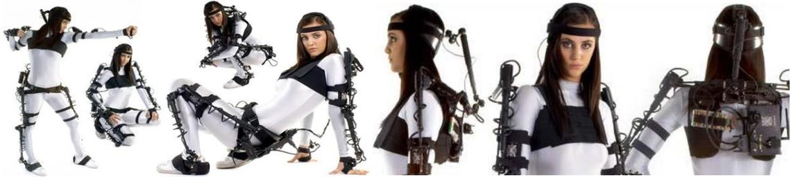
**Figure 7.** The Gypsy 6 mechanical motion capture suit. The Gypsy 7 has a resolution of 0.125 degrees [22] (Pictures from Pinterest.co.uk).
