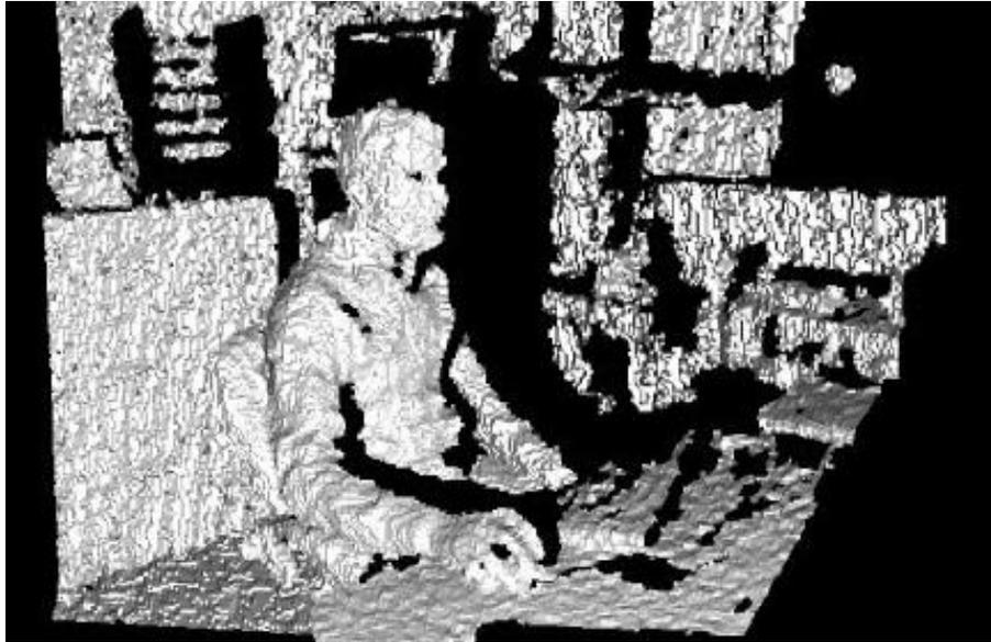
**Figure 3.** Kinect's 3D imaging abilities using specialized light patterns (Pictures from yting.com).
