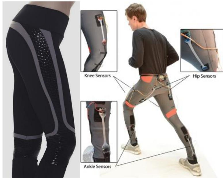
**Figure 9.** An example of a research, EAP, motion tracking suit (right, image from source [24]). Bend system (left, image from source [23]) claims to monitor knee flexion and glute “involvement,” which may mean sensing topical distortion caused by flexing gluts. The wearable soft sensing suit is a two-dimensional monitor, which still has linear calibration issues, possibly due to the participants’ inability to restrict themselves to pure planar motion.
