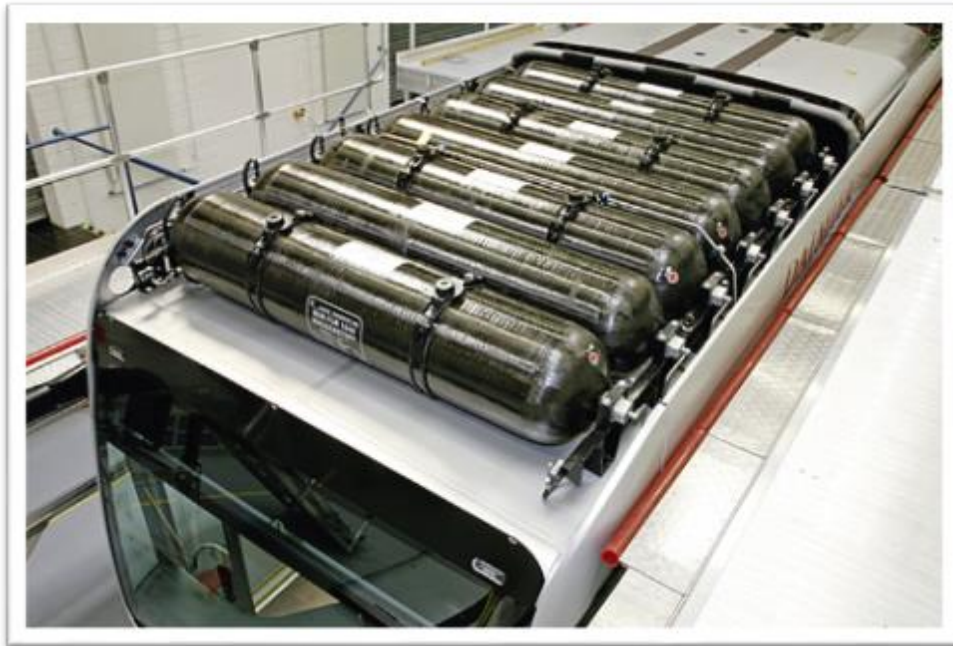
Figure 3. Hydrogen Storage System on Roof of Fuel Cell Bus
