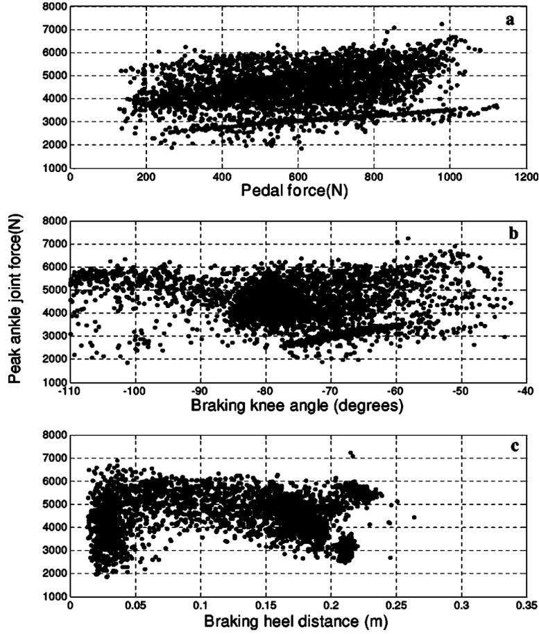
Fig. 6 Peak ankle force ( $F_{AJ}$ ) during the crash for all simulations and its relationship to BF (a), HD (b), and KA (c). HD is the distance of the heel from the toepan origin. KA equal to 0 deg signifies a full knee extension and  $-90$  deg signifies 90 deg of knee flexion.
