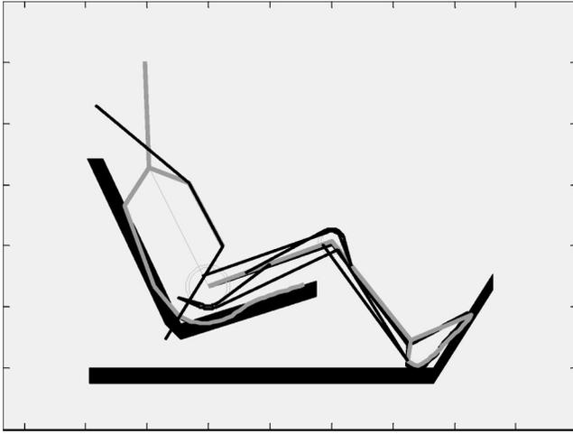
**Fig. 1** The seven body segments represented in the model (gray), the six muscles (black), the contact surfaces and the seat restraints. The passive left leg is resting on the toe pan and the active right leg is braking. The model is shown while braking prior to the crash with muscles at minimal activation and with a brake pedal force of 400 N.
