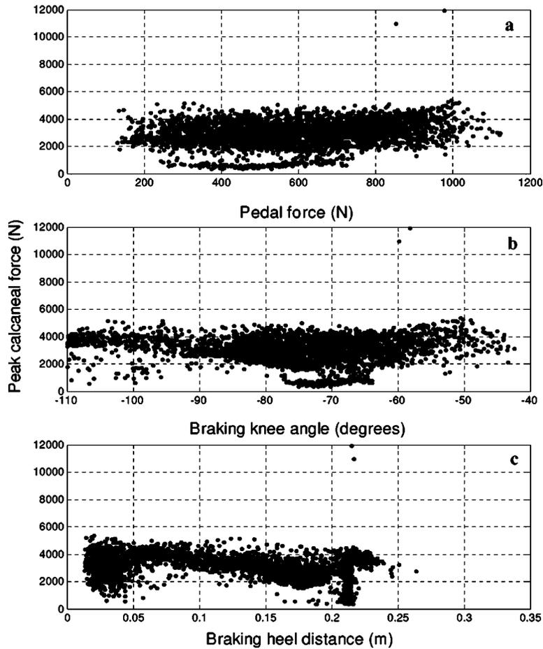
**Fig. 5 Peak calcaneal force ( $F_{CF}$ ) during the crash for all simulations and its relationship to BF (a), HD (b), and KA (c). HD is the distance of the heel from the toepan origin. KA equal to 0 deg signifies a full knee extension and  $-90$  deg signifies 90 deg of knee flexion.**
