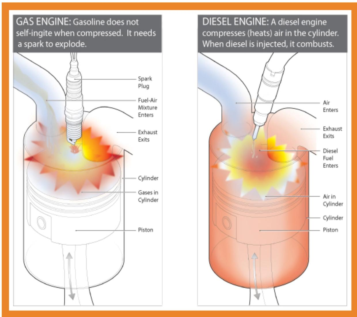
**Figure 2 – Gasoline-Spark versus Diesel Engine** Source: <http://ezibaco.vacau.com/gasoline-engines-vs-diesel-engines.php>
